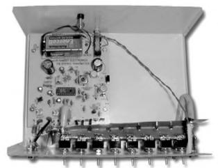
Figure 2 shows the schematic for a six-switch attenuator, for a still-optimistic total of 40dBf. Just change the resistor values in any of the  $\pi$ -filter sections to change the attenuation for that i tor to get the signal level at the tuner
