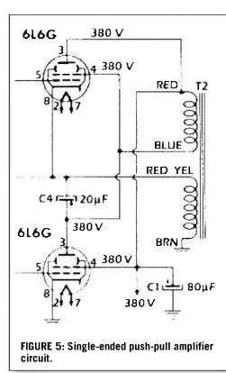
schematic, the top tube V1 is connected as a cathode follower and has no gain. The bottom tube V2 may have gain depending on its plate impedance in relation to the load. With equal drive you will usually get an asymmetric output.
