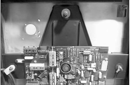
PHOTO 3: The turntable after removal of the Linn motor and power switch.
