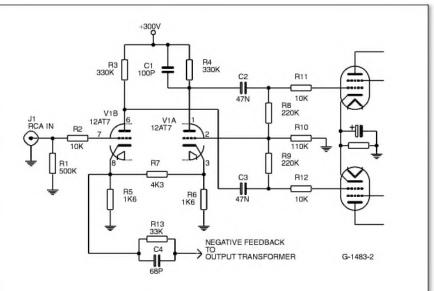
FIGURE 1: The new self-balancing inverter has better high-end performance characteristics than the old split-load inverter.
