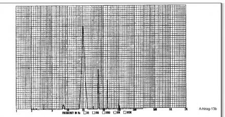
FIGURE 13(B): The same amplifier as in *Fig.* 13(A), but to which has been applied a rate of negative feedback of 6dB, which is, in effect, very little. Although the distortion rate has decreased, and although the bandwidth is slightly widened, one notes an apparent "compression" of the sound, a lack of aeration, of refinement (in the high notes). Note that the harmonics of high order have disappeared, absorbed by the feedback loop.
