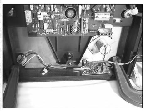
PHOTO 4: Completed modification showing speed/power switch at left, the speed control board, and the motor. The DC power wires are arranged to exit the base at the right.
