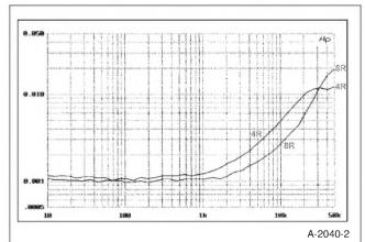
FIGURE 2: The distortion roughly doubles due to LSN as loading increases from 8 to  $4\Omega$ , using modern output devices such as MJ15024/25. (NB: The  $4\Omega$  THD is less than the 8 $\Omega$  above 30kHz solely due to fortuitous cancellation of harmonics.)
