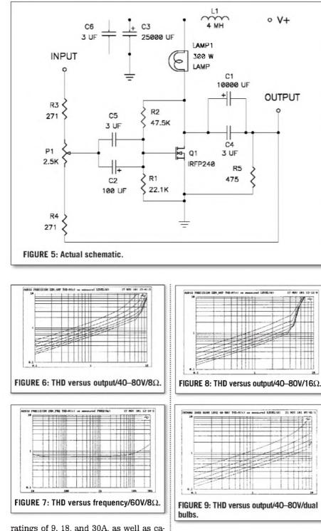
ratings of 9, 18, and 30A, as well as capacitances of 600pF, 1,300pF, and 2,600pF, respectively. These figures are proportional to chip size, and from actual testing you'll get similar performance from two IRF230s in parallel as compared to a single IRF240. Also, the IRFP250 behaves similarly to a pair of IRF240s.
