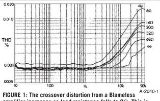
amplifier increases as load resistance falls to  $8\Omega$ . This is not due to LSN. (All THD plots are taken at 80kHz bandwidth, RMS sensing.)
