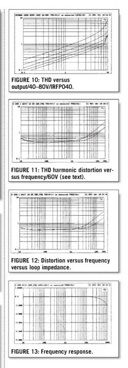
The lower voltage chips of the same type will give lower distortion, apparently due to their lesser sensitivity to voltage fluctuations on the Drain. They are generally the preferred parts.
