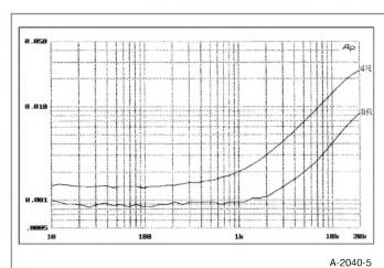
FIGURE 5:  $4\Omega$  distortion is three times greater than  $8\Omega$  for the venerable 2N3055/2955 output devices. Compare *Fig. 2*.
