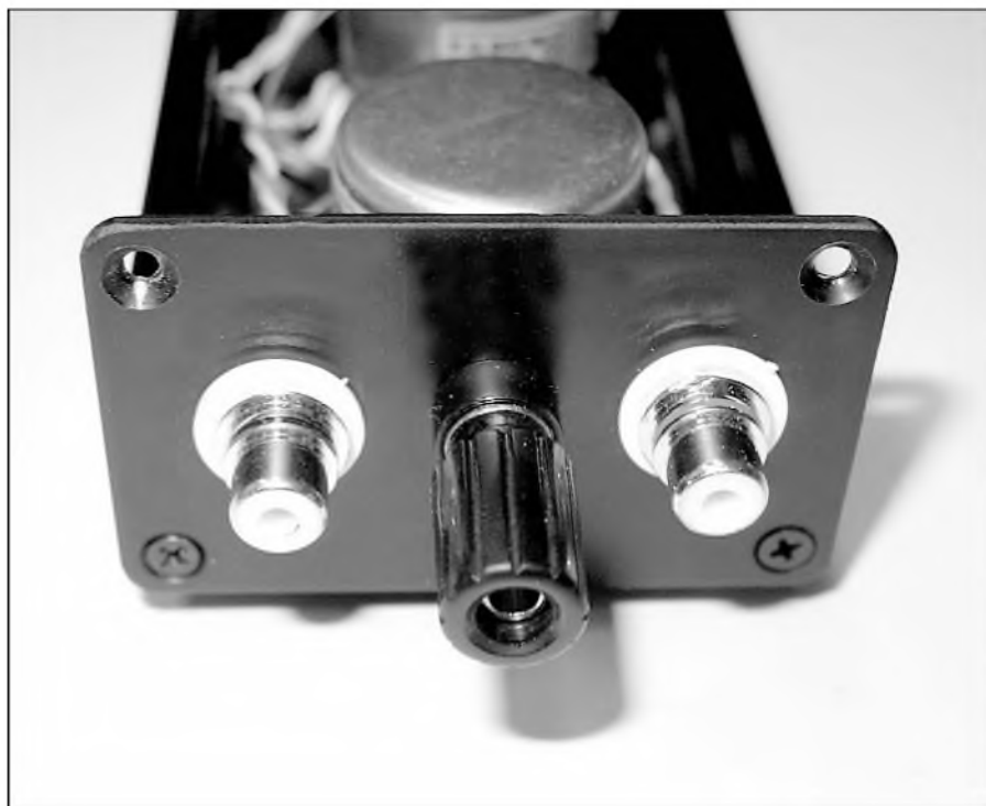
PHOTO 8: The RCA jacks and ground binding posts.
