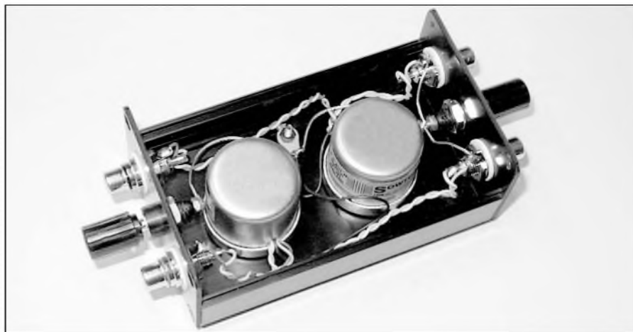
PHOTO 6: The transformers mounted into an aluminum enclosure.
