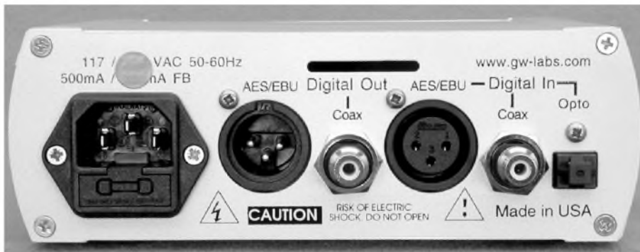
PHOTO 2: The rear panel features Toslink Optical plus AES/EBU and S/PDIF inputs, along with AES/EBU and S/PDIF outputs.
