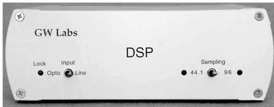
PHOTO 1: Front view of the GW Labs DSP. Two switches select line or opto inputs, and an output sampling frequency of 44.1 or 96kHz.
