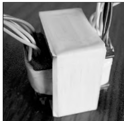
PHOTO 3: A moving-coil transformer shown outside of its metal case (courtesy Sowter Company).
