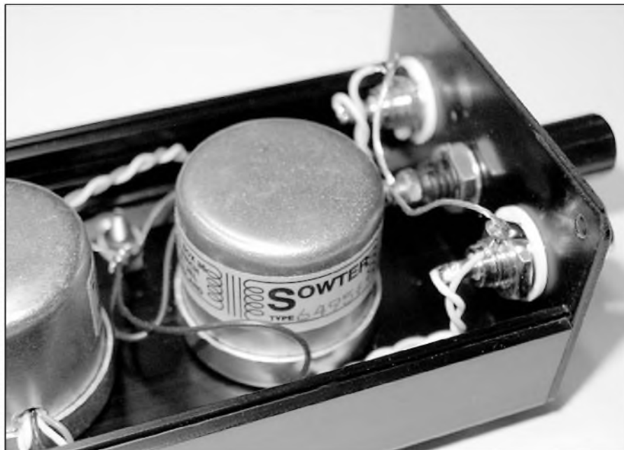
PHOTO 7: Close-up of the input jacks. Note the extra ground wire run to the RCA jacks (see text).
