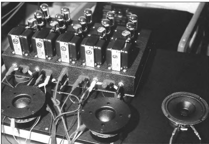
PHOTO 6: Amplifier under test with speakers connected to all five channels. (Three are visible and the other two are mounted under workbench.)
