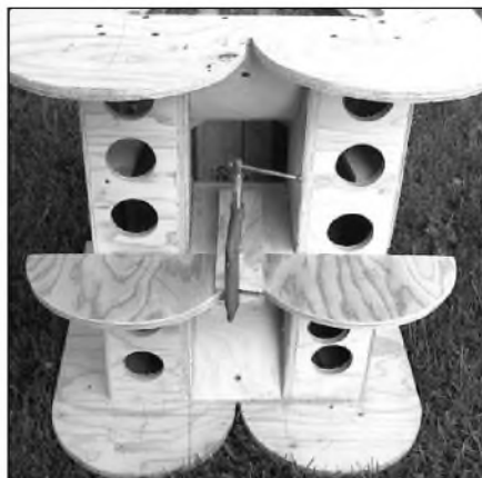
PHOTO 16: Holding back braces in place while hot-melt glue sets.
