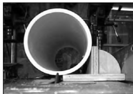
PHOTO 17: Using a jig to secure PVC pipe for cutting.
