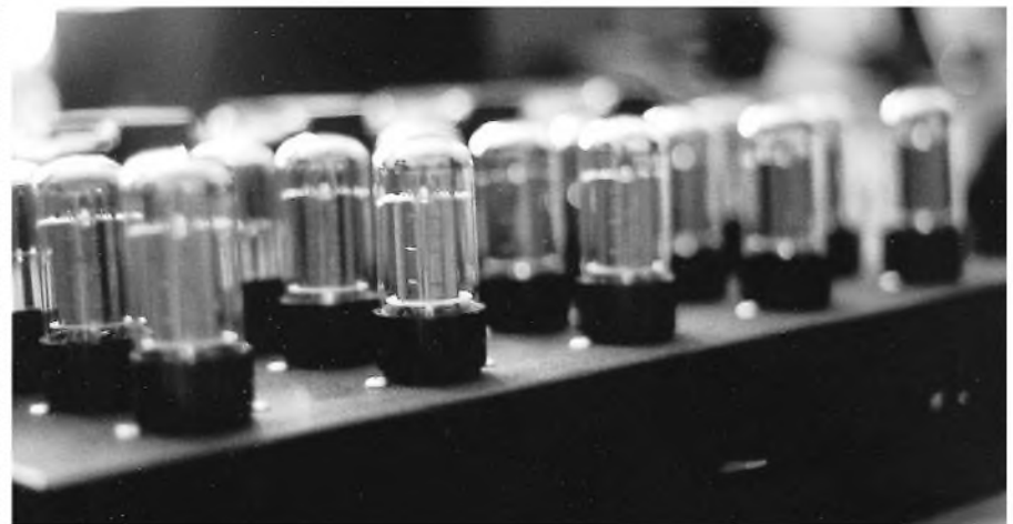
PHOTO 1: Amp in operation with 15 glowing valves (three for each of the five channels).
