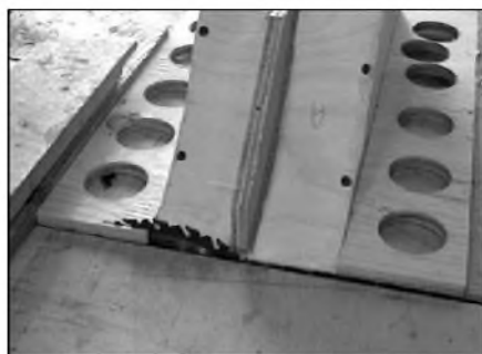
PHOTO 6: Trimming the throat horn and supports on the table saw with panel cutting jig.
