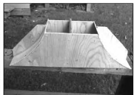
PHOTO 4: Completed throat horn. Note how cauls are now braces.
