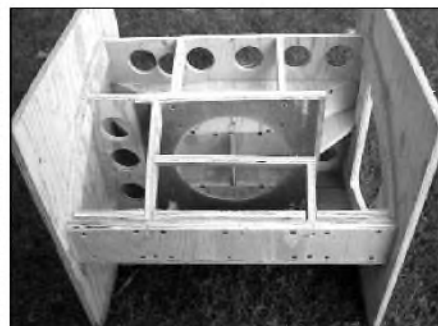
PHOTO 11: Assembly after installing horn braces.
