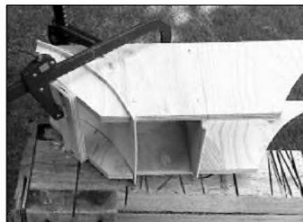
PHOTO 3: Attaching throat horn sheathing using clamps and cauls.
