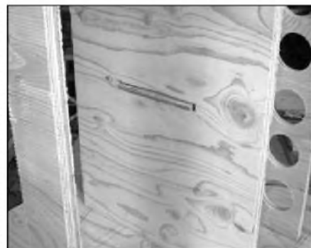
PHOTO 9: Determining the baffle hole location.
