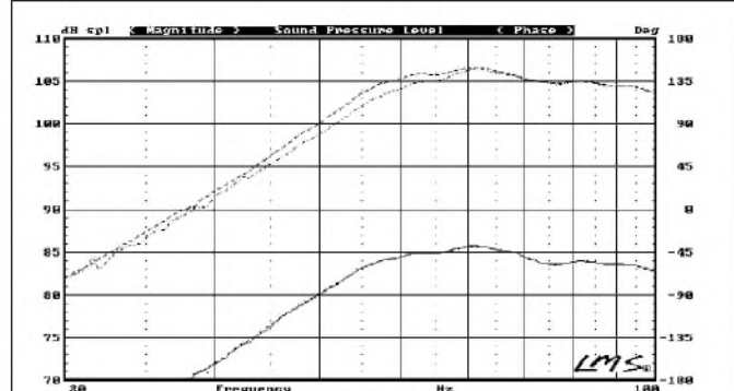
FIGURE 6: Sound pressure level (SPL) comparison of 9½" flared port against 8½" straight port at 1.00V and 11.32V. Flared port SPL is the top trace at both power levels.
