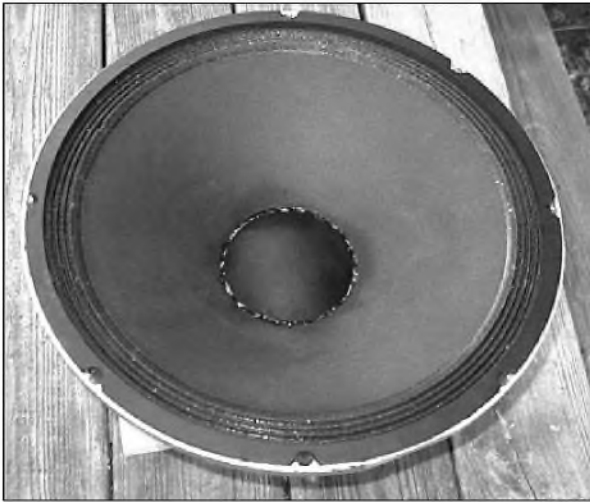
PHOTO 8: The finished reconed driver.
