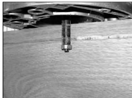
PHOTO 16: Router bit with guide bearing below the cutting edge.
