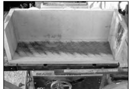
PHOTO 11: Dry-assembling the box parts.
