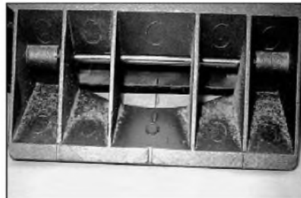
PHOTO 9: Setting the biscuit cutter shoe at the joint center mark.
