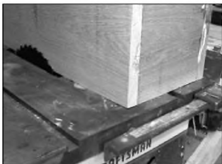
PHOTO 14: Setting the fence with the box to cut the baffle to size.
