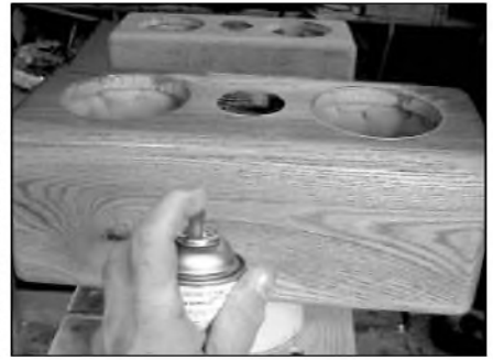
PHOTO 23: A final coat of spray urethane is easier to apply with the box atop a lazy Susan.
