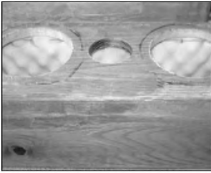
PHOTO 21: Driver holes are cut before sanding filler.
