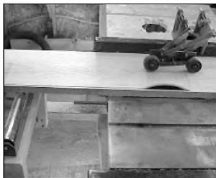
PHOTO 6: Cutting a board to finished width.
