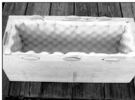
PHOTO 15: Lining the box with foam before attaching the baffle.
