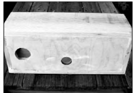
PHOTO 13: Holes in the rear of the box for port and wiring cup.
