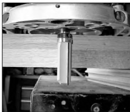
PHOTO 5: A router bit with guide bearing above the cutting edge.
