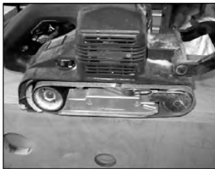
PHOTO 17: Rough-sanding with a belt sander.
