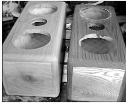
PHOTO 22: Before and after applying oil-base urethane.
