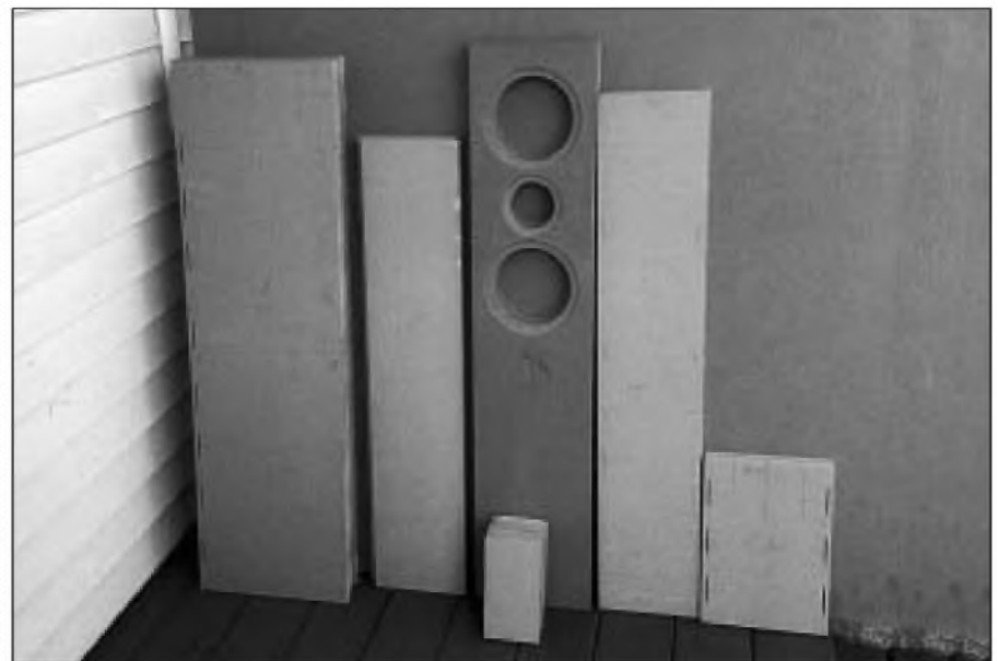
PHOTO 1: THOR enclosure parts are cut out. From left they include the sides, baffle boards, front panels with angle blocks below, back panels, and tops.
