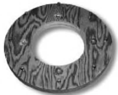
PHOTO 11: Readying plywood ring for mounting.
