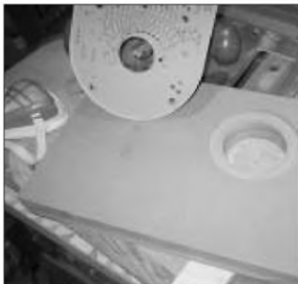
PHOTO 5: A test cut for the tweeter hole, showing the Jasper rig and the dust mask.
