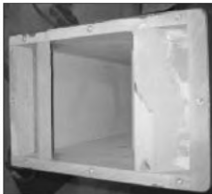
PHOTO 11: Bottom side of the tower showing the angled blocks and the brass inserts installed. Note that I used Mortite between the angled blocks and the back and front panels, to seal any void.
