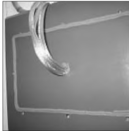
PHOTO 13: Top of the base. After taking the photo I removed one row of Mortite to avoid more overkill. Speaker wires are sealed with hot-melt glue.
