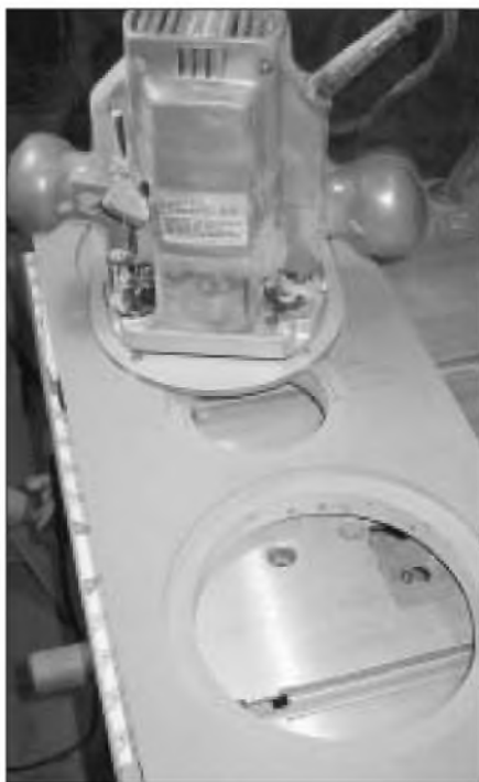
PHOTO 6: The plunge router and Jasper guide do a good job of cutting holes and rim recesses.
