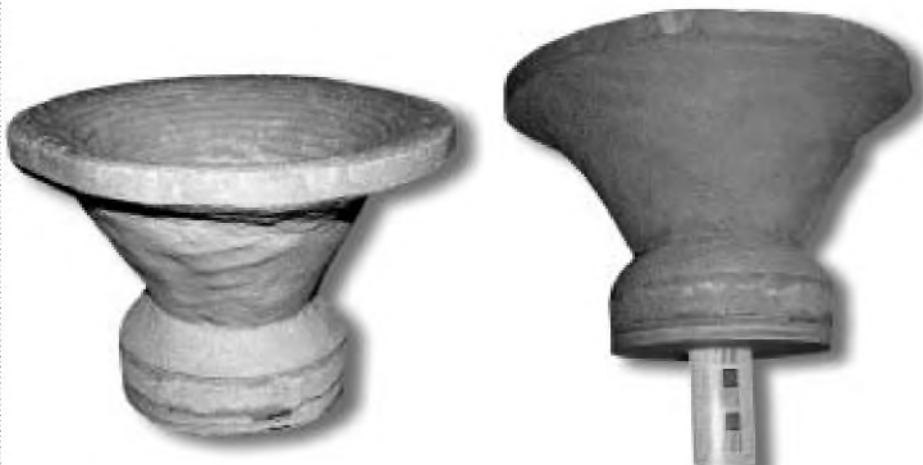
PHOTO 5: The author's first horn (12" diameter, with 2 1/4" diameter throat).
