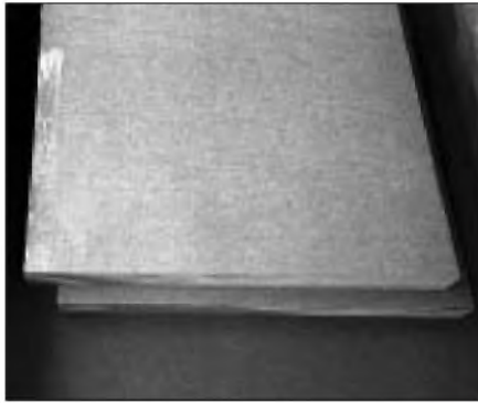
PHOTO 2: Closeup of the baffles showing the 86° angle cut.
