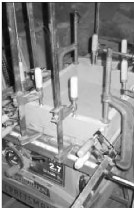
PHOTO 9: Even the simple five-part base requires more clamps than you anticipate.
