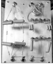
PHOTO 2: Component layout. The circuitry on the left is the low-pass. The high-pass circuitry is on the right. I used a bus wire ground for each section, even though the RCA jacks are mounted to the cover.
