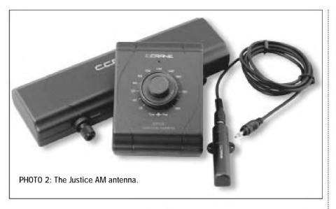
supply. It is contained in two "black boxes" about the size of an outstretched hand (*Photo 2*). One box is the "head," containing the tuning coil plus sophisticated circuitry on a PC board. The other box contains the two concentric tuning knobs (coarse and fine) plus the special power-supply circuit.
