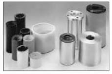
PHOTO 2: Some of the many types of mandrels used with the Pengelly-Stringer Mk. 3 are shown on the left. These will accommodate a wide variety of cylinder records, shown on the right. (Courtesy of Joe Pengelly)
