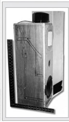
PHOTO 2: Markings on side of cabinet show internal baffles of transmission line bass portion with 8" woofer. I stuffed the TL with polyester fiberfill from a discarded bed pillow. Midrange section on top is open to rear dipole style. To minimize diffraction, I covered the front with plastic foam and rounded all edges with a router.
