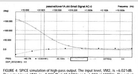
The output level, VM1, is -0.085dB at 40.179Hz and +6.002 at 1000Hz. The actual circuit measured within  $\pm 0.2$ dB.
