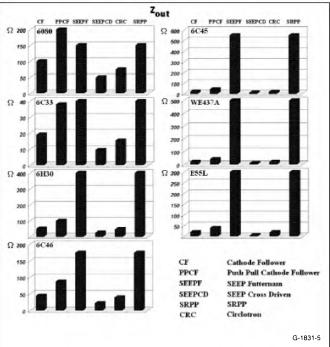
FIGURE 5: The output impedance Z<sub>out</sub> for standard OTL output stages in various triodes.
