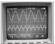
PHOTO 7: 12FM6, 19V bias, 1V RMS out (top) and distortion residual (bottom).
