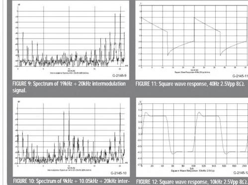
The 12Vpp output test level for a multi-tone intermodulation signal (MIM, Fig. 10) of 9kHz + 10.05kHz + 20kHz produced a 1kHz response product of 0.89%. I also plotted the 1kHz product of this MIM signal versus output power in Fig. 2. This gives a better indication of the K12M's nonlinear response, since it is a closer approximation to music than a sine wave.
