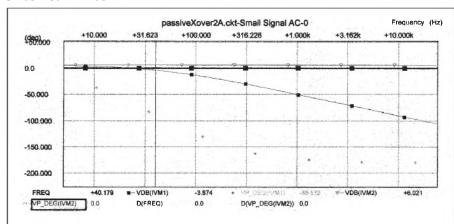
FIGURE 3: SPICE simulation of low-pass output. The input level, VM2, is +6.021dB. The output level, VM1, is -3.874dB at 40.179Hz and +2.15 at 16Hz. The actual circuit measured within  $\pm$ 0.2dB.
