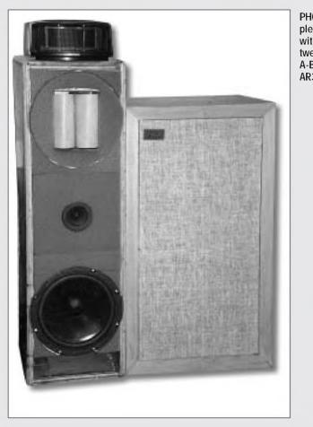
PHOTO 3: Completed speaker with Linaeum tweeter ready for A-B test versus AR3a. Using sheet metal, I fashioned the front baffle, to which I fastened the free ends of the diaphragm (*Photo 2*). *Photo 3* shows this midrange speaker in a TL enclosure. The back of the midrange is open to the rear.
