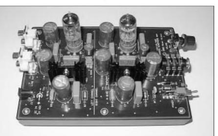
PHOTO 1: The low-voltage hybrid headphone amp.
