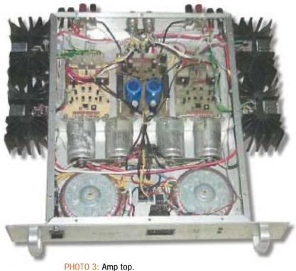
with the kit for the Hitachi transistors, and these are not adequate for class A operation at the 100W/channel output level, this amplifier was intended to be operated class AB. Thus, based on the observed distortion behavior, the bias current for the output MOSFETs was increased until I observed little improvement in THD. This was achieved with a drain current of about 130mA, a value that squares with Erno Borbely's recommended value for these devices of 100mA.<sup>9</sup>
