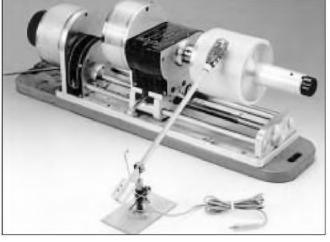
PHOTO 1: The Pengelly-Stringer Mk. 3 Phonograph, used to transfer the cylinder recordings on Sounds Cylindrical. The straight, pivoted tonearm and moving-mandrel design ensure low tracking error and minimal record wear. (Courtesy of Joe Pengelly and Bill Klinger)
