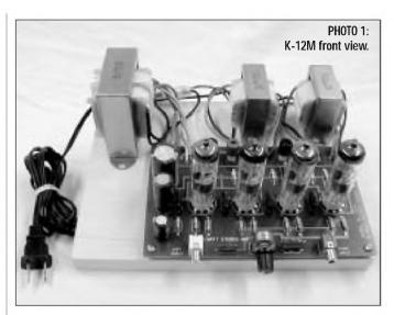
6mm nylon spacers and the aforementioned screws. Ceramic tube sockets hold the four tubes.
