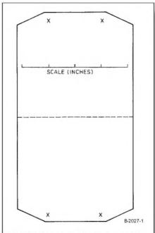
FIGURE 1: Pattern for diaphragm cut from drum head. Fold 180° at dotted line. Punch holes approximately ¼" at Xs.
