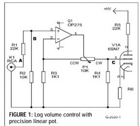
following attenuation. This results in a gain of +20dB between points B and C. In full counterclockwise position the gain of Q1 is  $1\times$ , but is followed by an attenuation of (10 + 1.1):  $1.1 = 0.1\times$ , giving a gain of -20dB between points B and C.
