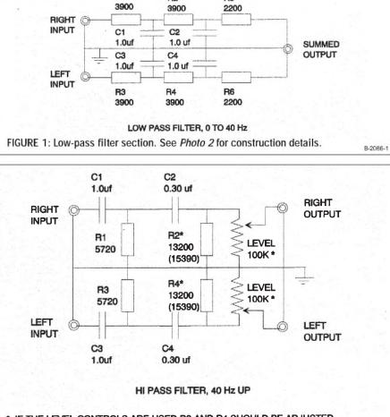
\* IF THE LEVEL CONTROLS ARE USED R2 AND R4 SHOULD BE ADJUSTED AS FOLLOWS; RIN = THE INPUT RESISTANCE OF THE AMPLIFIER.
