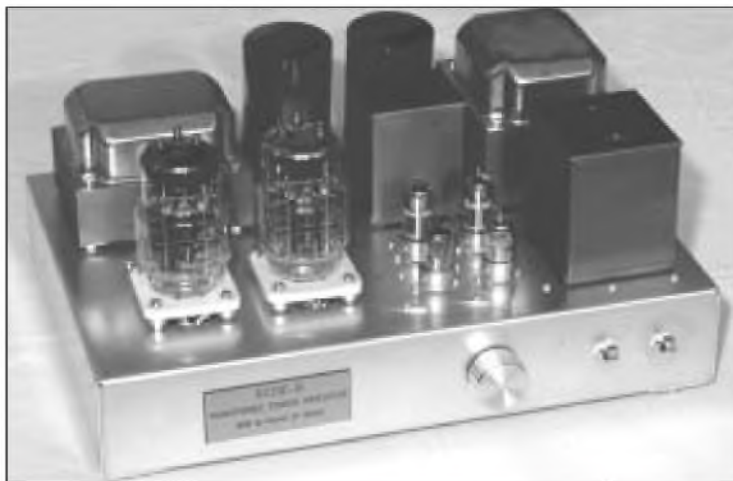
PHOTO 1: The revised 6C33C-B power amp.
