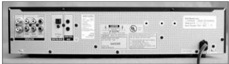
PHOTO 2: Rear view of the SCD-CE775. The stock PC-mount RCA jacks for the two-channel outputs are replaced with Cardas GRFA connectors by SACDmods.
