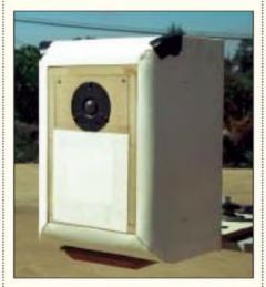
PHOTO 5: Test enclosure with 2" radius shell.
