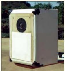
PHOTO 6: Test enclosure with 1" radius shell.
