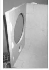
PHOTO 4A: Biscuits in place on inner face of the front panel with mated side and bottom.
