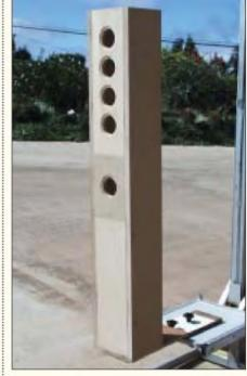
PHOTO 3: A test enclosure that is 8.875" wide and 56" tall.
