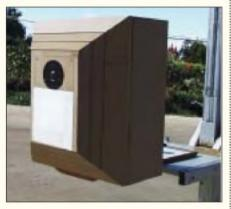
PHOTO 7: Test enclosure with 4", 45° bevel shell.
