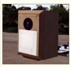
PHOTO 9: Test enclosure with 1", 45° bevel shell.
