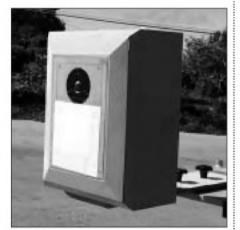
PH0T0 10: Test enclosure with dual bevel,  $22^{\circ}$ ,  $45^{\circ}$  shell.
