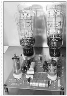
PHOTO 2: Testing THD with VV30 power triodes.
