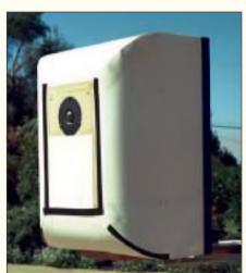
PHOTO 4: Test enclosure with 4" radius shell.
