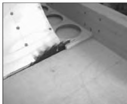
PHOTO 8: Trimming and squaring with the panel-cutting jig.
