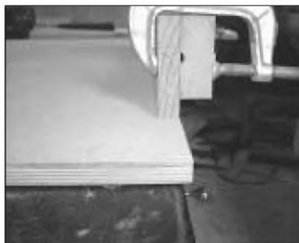
PHOTO 6: Reinforcing the push-bar.
