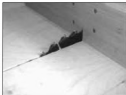
PHOTO 7: The blade passes through the lowermost portion of the push-bar.
