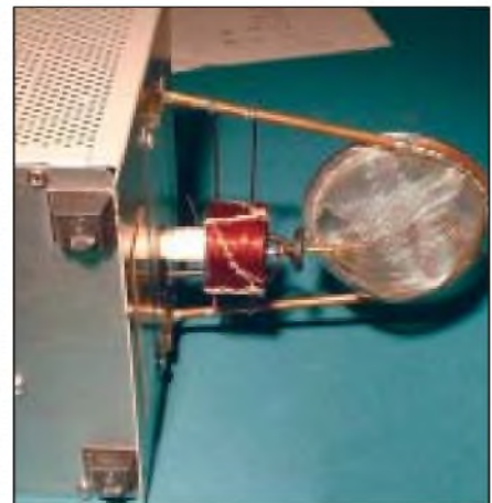
PHOTO 4: Resonant coil, little feedback loop, and Faraday shield.
