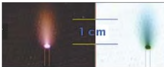
PHOTO 2: The corona discharge on the electrode (left); shown with inverted colors (right).
