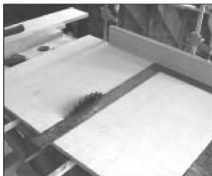
PHOTO 5: Squaring the push-bar to the blade.
