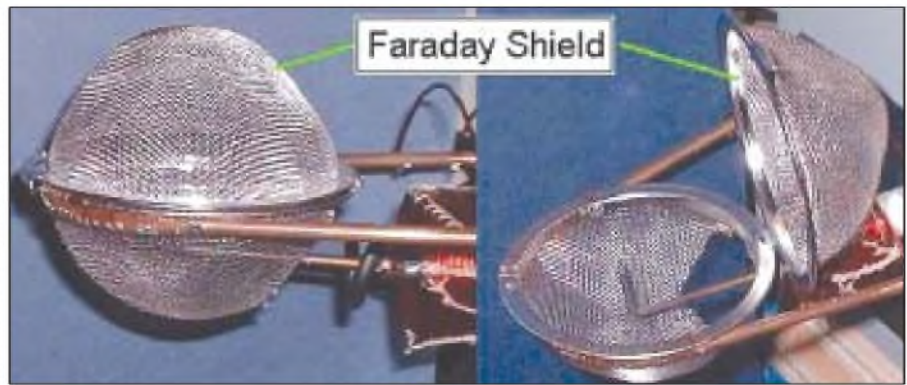
PHOTO 3: The Faraday shield is simply a food strainer.
