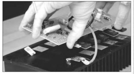
PHOTO 3: Removing the original PC board.
