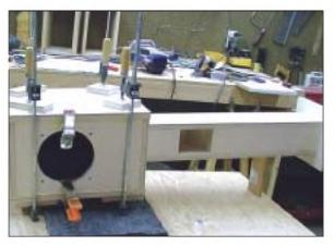
PHOTO 11: Gluing on the box sides. 14 audioXpress 6/03
