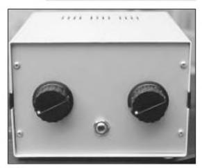
PHOTO 2: The final version of the headphone amplifier in a metal cabinet. I used separate volume controls for each channel rather than a dual Alps pot since I like to make occasional small adjustments of channel balance.
