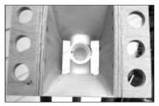
PHOTO 10: PVC "T" glued into the horn throat.
