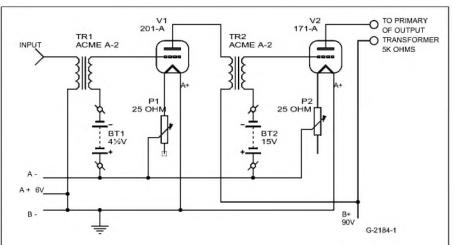
FIGURE 1: This is the circuit of the 1920s style amplifier. It sounds great playing '20s music. Note the filament and bias connections: the positive side of the bias batteries go to A– while A+ is connected to B–. I explain the reasons for this in the text.
