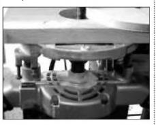
PHOTO 14: Trimming radiused parts with a table-mounted router.
