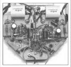
PHOTO 10: PTP board assembled.
