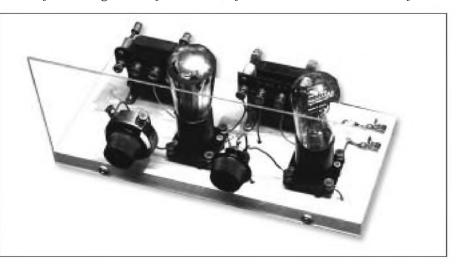
PHOTO 2: A re-creation of a 1920s style audio amplifier that might have been found in most American homes. A 201-A and a 171-A are mounted on a  $12 \times 5''$  board, with a Plexiglas panel. The transformers and most other parts are from the '20s.
