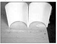
PHOTO 13: Tracing PVC halves onto cabinet top and bottom.
