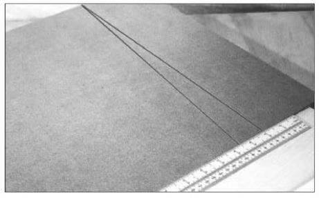
PHOTO 9: A scale and a calculator will give you more accurate angles than a line protractor.
