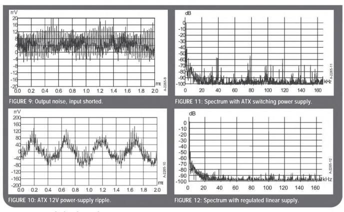
output stage, overlaid with switching supply noise. THD+N at this test point is 0.26%.
