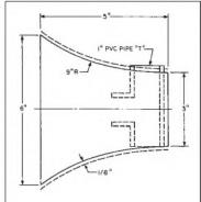
FIGURE 3: Throat horn side view.
