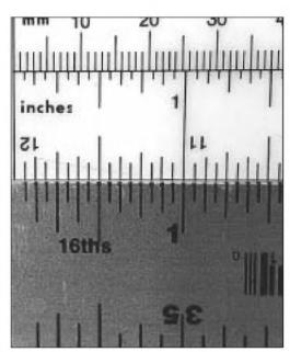
PHOTO 1: The shadow makes this look worse than it is, but the first sixteenth on the bottom scale is more like  $\frac{5}{32}$ , making the scale unusable from the end.
