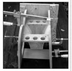
PHOTO 18: Using clamps to align parts before screwing in place.
