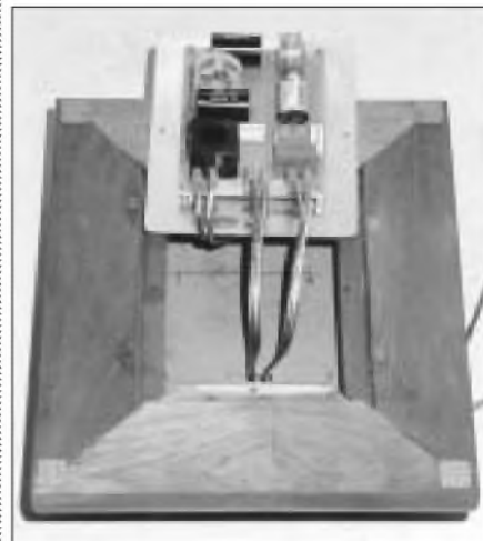
PHOTO 7: Crossover view before installing onto the base.
