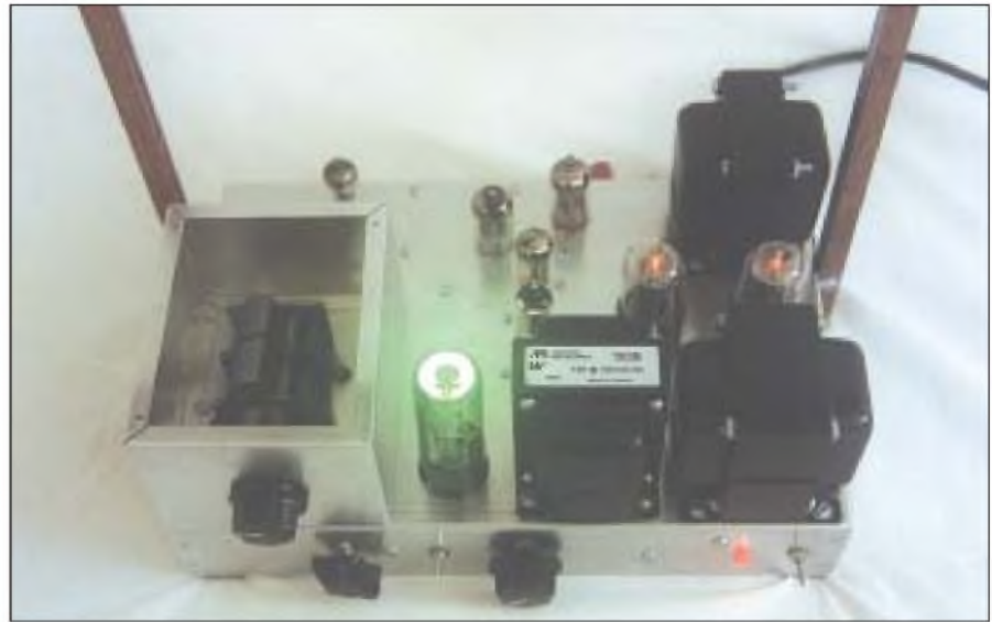
PHOTO 1: Front view of the radio receiver. The RF circuits are on the left, with tubes V1 and V2 at the left rear.
