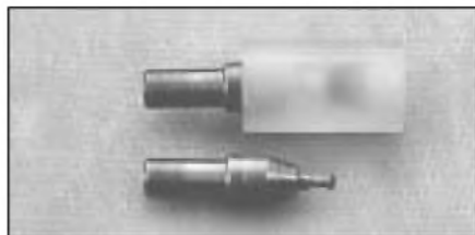
PHOTO 4: Electrode inserted in a cell. The second electrode is for reference to illustrate the relative position of the parts of the electrode inside the cell.
