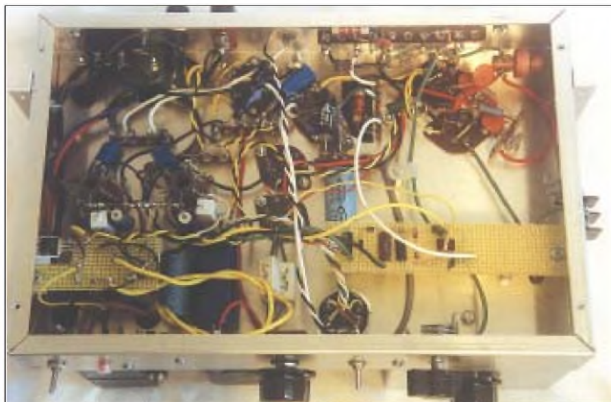
PHOTO 4: Underside view of the chassis. The RF wiring is at the right rear.
