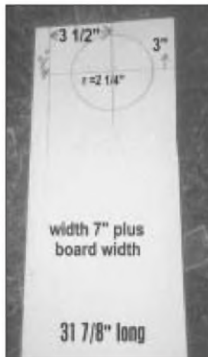
PHOTO 1: All sides of this project are the same. Since the material is 3/4" thick, the side boards are just over 7 3/4". The driver needs an opening of radius 2 1/4".
