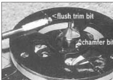
PHOTO 2: The chamfering bit used to widen the inside of the opening. Resting on the router is the flush trim bit used after assembly.
