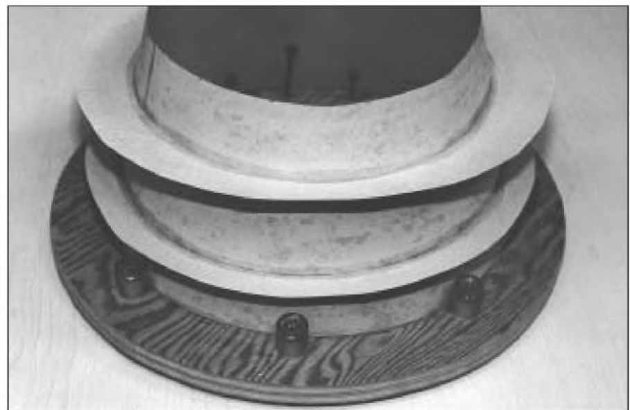
PHOTO 5: Fitting the base retainer mold sections, reinforced by a second ring.
