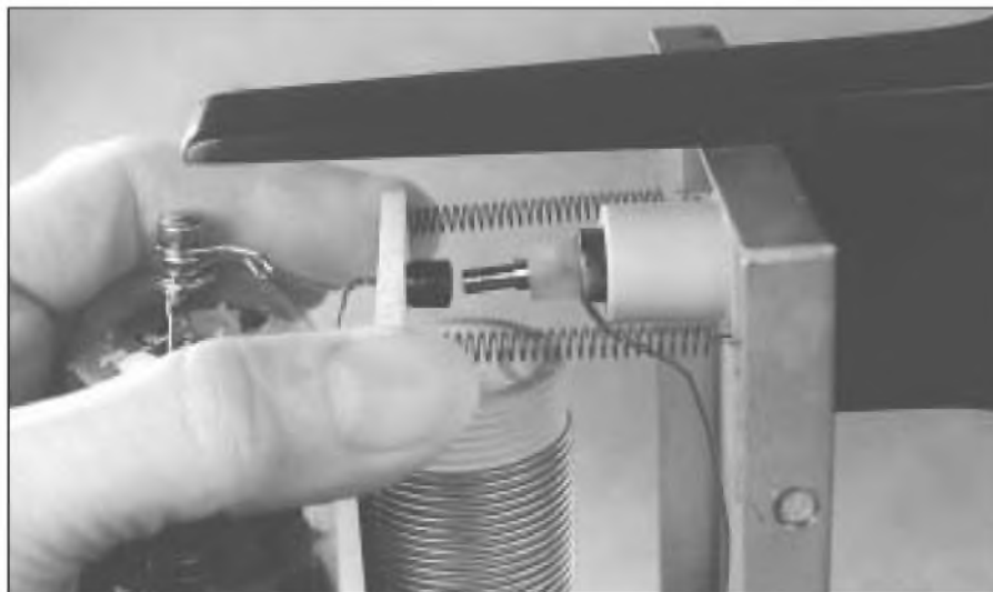
PHOTO 7: The correct way to hold the ceramic bar for removal of the cell components.
