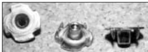
PHOTO 4: "T-nuts" used to reliably install the speakers.
