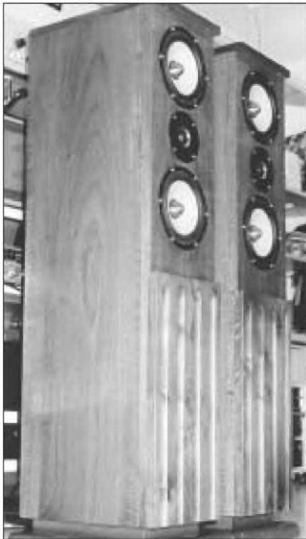
PHOTO 1: Overall towers view. You can see the provision made to accept the grille frame once ready. I'm thinking of using thin material similar to ladies' elastic stockings.
