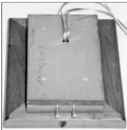
PHOTO 6: A view of the base. You can see the wires coming through the panel before sealing the hole with silicon glue. Also visible are the golden speaker's terminals.
