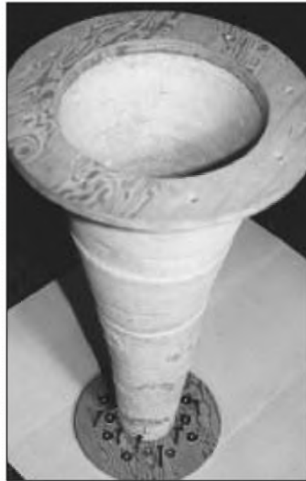
PHOTO 11: Aligning the wooden and concrete throats.
