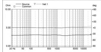
FIGURE 19: Predicted impedance of Vifa XT-25 with calculated Zobel network.
