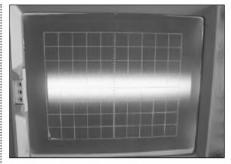
PHOTO 5: Battery noise scope ( $10\mu V/div$  RTI, 2ms/div, 4.9 $\mu V$  RMS).
