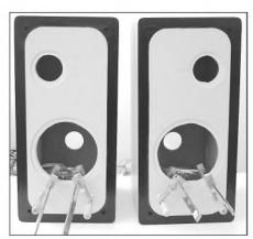
PHOTO 8: Clamping woofer opening interior braces
