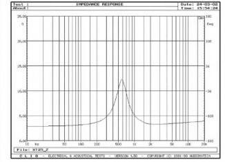
FIGURE 18: Impedance plot for Vifa XT-25.
