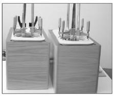
PHOTO 9: Completing clamping the front panel braces in the woofer area.
