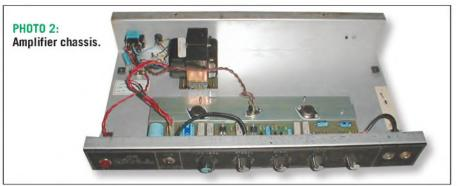
measurements on the amplifier (Fig. 2), and it puts out only 30W at 3% THD, 1kHz into  $4\Omega.$  The power supply rails drop from  $\pm 37V$  DC NL to  $\pm 28V$  at maximum load,  $4\Omega.$  At 41Hz, it makes 43W into  $8\Omega$  and 28W into  $4\Omega,$  3% THD. The power transformer looks a bit small, putting this unit into the "practice amp" category.
