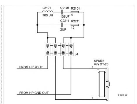
FIGURE 22: Tweeter Zobel board network, connected between HP network and tweeter (note tweeter polarity).
