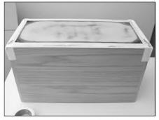
PHOTO 5: Masked and sanded, ready for attaching front panel build-up.
