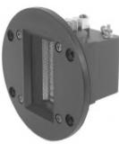
produce sound. In an aluminum ribbon tweeter, the ribbon itself is both the conductive material and the radiating mass moved by the magnet to produce sound. This method results in a wider band width and very smooth phase response. At 0.011 grams, the pure aluminum ribbon has a mass of about 1/20th that of a dome tweeter with comparable surface area.
