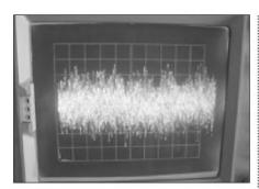
PHOTO 9: HP6236B supply noise scope  $(500\mu V/div\ RTI,\ 2ms/div,\ 340\mu V\ RMS)$ .
