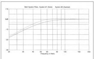
FIGURE 12: Box design software plot of QX108 actual versus measured data.
