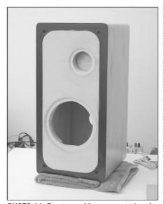
PHOTO 11: Front panel braces routed and tweeter sub-baffle installed.
