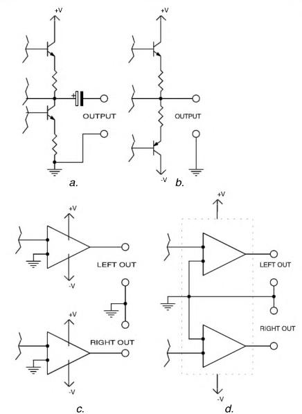
FIGURE 3: Typical power output circuits for bipolar junction transistor (BJT) audio amplifiers. a. Quasi-complementary symmetry (QCS); b. Full-complementary symmetry (FCS); c. Discrete integrated circuit (DIC); d. Combined integrated circuit (CIC).
