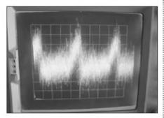
PH0T0 8: LM340/LM320 supply noise scope (100 $\mu$ V/div RTI, 2ms/div, 105 $\mu$ V RMS).
