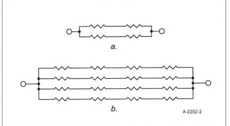
FIGURE 2: Practical 8 $\Omega$  load resistor networks for audio power testing. a. 80W load; b. 320W load. All resistors are 8 $\Omega$ /20W 5% non-inductive (see text).
