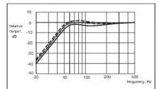
FIGURE 17: Effects of loudspeaker Q. (From top to bottom, the curves represent  $\mathbf{Q}_{TS}=0.52,\,\mathbf{Q}_{TS}=0.4,\,\mathbf{Q}_{TS}=0.28;$  for all curves,  $\alpha=0.7,\,h=1,$  and  $\mathbf{Q}_{L}=7.)_{_{B-2233-17}}$
