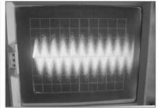
PHOTO 10: Galo supply noise at 20kHz scope (100 $\mu$ V/div RTI, 50 $\mu$ s/div, 68 $\mu$ V RMS).
