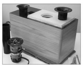
PHOTO 13: Back panel after routing for port mounting flare.
