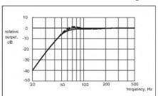
FIGURE 18: Effects of box Q. (From top to bottom, the curves represent  $Q_B=9.8$ ,  $Q_B=7$ ,  $Q_B=4.9$ ; for all curves,  $\alpha=0.7$ , h = 1, and  $Q_{TS}=0.4$ .)
