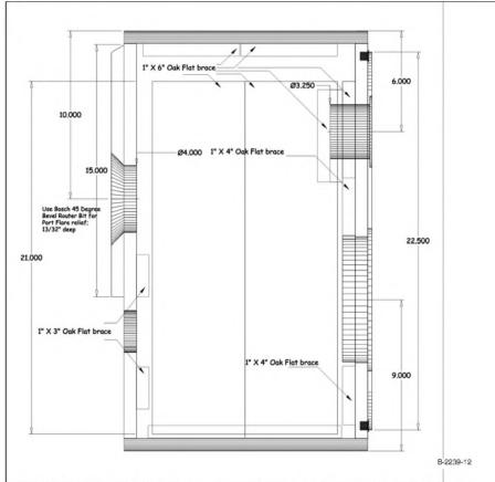
FIGURE 12: Side construction view of modified Woodstyle enclosure with dimensions.
