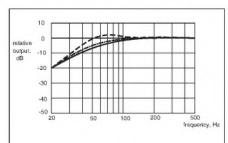
FIGURE 13: Frequency responses for sealed cabinets of different sizes.
