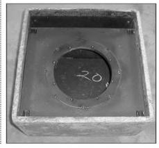
PHOTO 6: Adapter ring installed and painted, Tolex removed.
