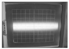
PHOTO 4: Noise meter amp scope, input open ( $10\mu V/div RTI$ , 2ms/div,  $4.7\mu V RMS$ ).
