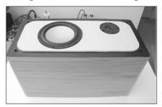
PHOTO 7: Checking driver fit after cutting holes.
