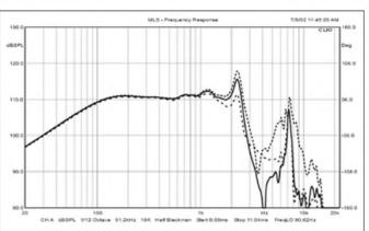
FIGURE 17: Near-field measurements of M8a at center, mid to edge, and edge near surround.
