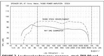
FIGURE 7: Loudspeaker frequency response, stock TKO 80 and NHT SW2.
