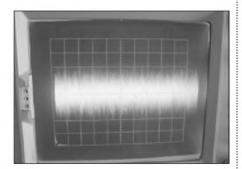
PHOTO 7: Galo supply noise scope (100μV/div RTI, 2ms/div, 42μV RMS).
