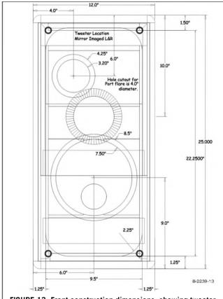
FIGURE 13: Front construction dimensions, showing tweeter and woofer locations (mirror right and left), with front panel build-up using  $\frac{1}{4}$  HDF.
