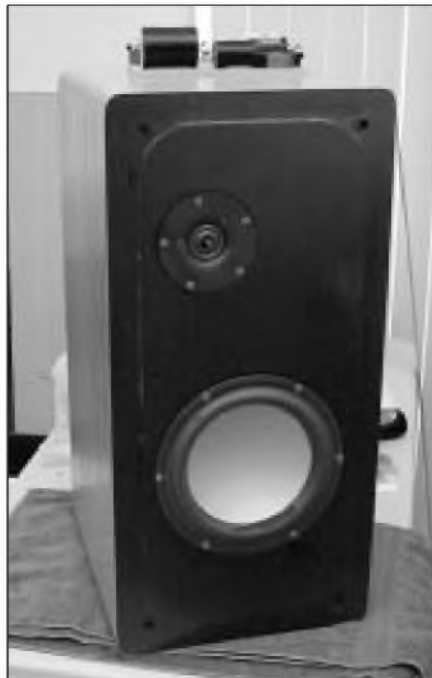
PHOTO 25: Enclosure for first tests, without diffraction control treatments.
