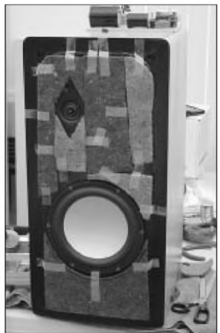
PHOTO 26: Testing felt layout for diffraction reduction.
