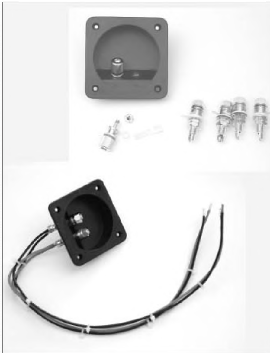
PHOTO 23: Input cup with new binding posts.
