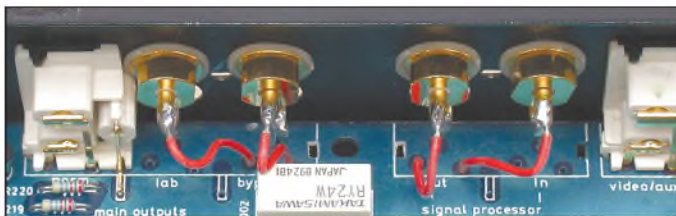
PHOTO 3: New RCA output connectors. The pair on the right are an optional set of aux outputs that may be useful for biamping. The "norm" output jack block, cut away from the original three-pair assembly, has no electrical function, but it supports the corner of the PC board.
