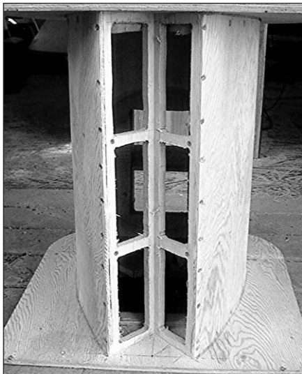
PHOTO 15: Tweeter holes completed.
