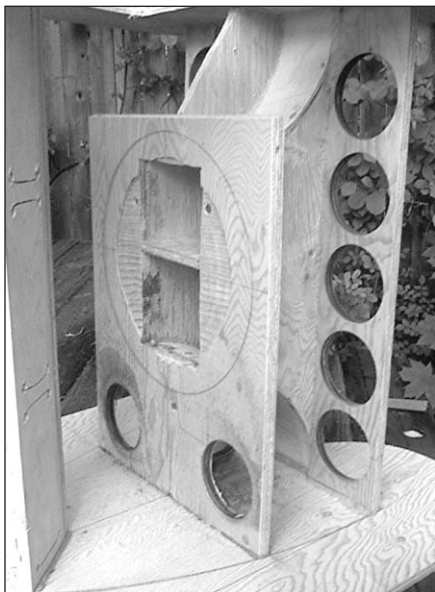
PHOTO 9: Baffle in place.
