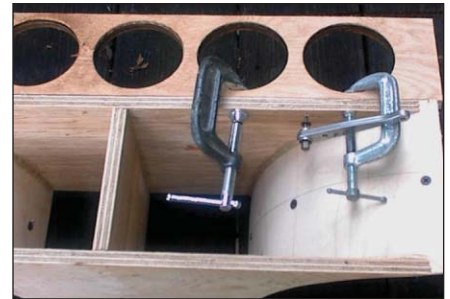
PHOTO 5: Attaching throat horn supports.
