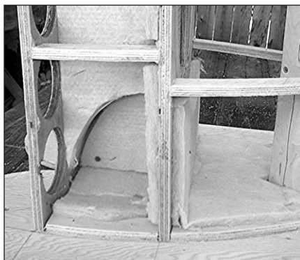
PHOTO 12: Lining with damping fiberglass.
