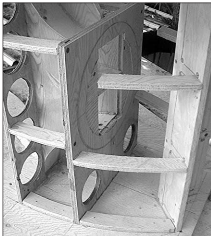
PHOTO 10: Horn braces. Note the "incomplete" brace.
