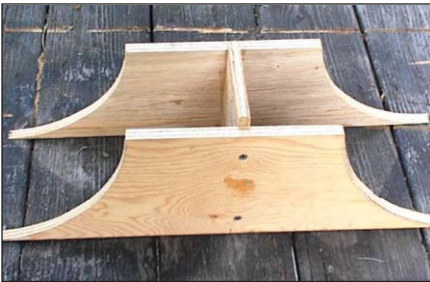
PHOTO 2: The throat horn sides and divider.
