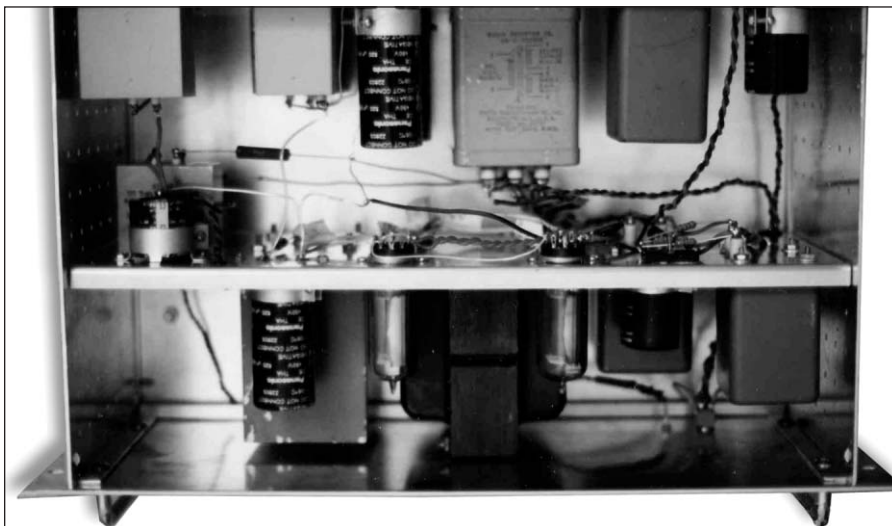
PHOTO 3: Power supply. Front of preamp is at the bottom of photo (author's note: note rack handles at front!).
