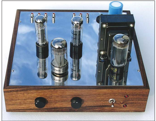
PHOTO 1: Top view of low-mu triode preamp.
