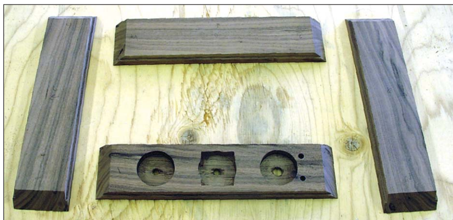
PHOTO 6: Wood for base, cut and ready for assembly.
