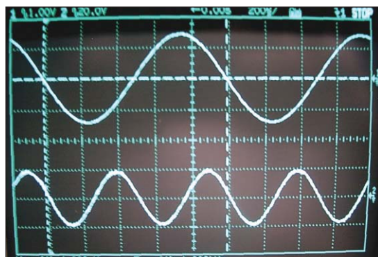
PHOTO 11: Output (top) and distortion residual (bottom, not to scale).
