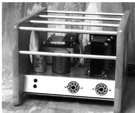
PHOTO 2: Separate power supply constructed similarly. High voltage 300V DC.
