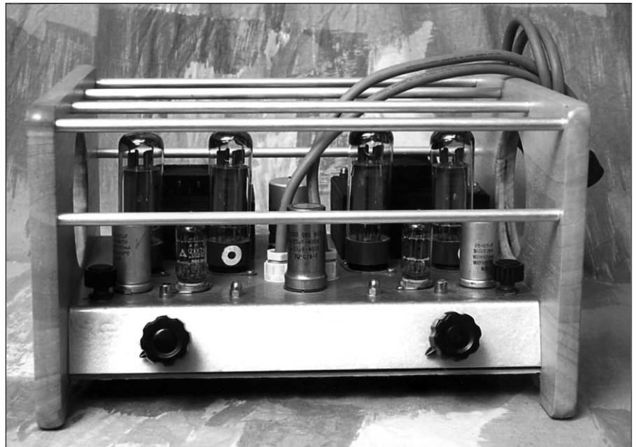
PHOTO 1: Two channel 15W/channel, ultralinear with a separate power supply. The chassis is U-shaped aluminum with wood end pieces held together with internally threaded aluminum rods.
