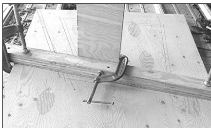
PHOTO 3: Attaching the first horn plate to a side.
