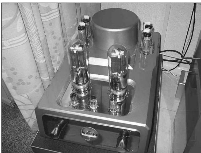
PHOTO 1: Front view of the ALFI PSE monoblock amplifier HQSE 65. You can see the special table made for these 35kg monoblocks. The weight is due, for the most part, to the giant power transformer and the van der Veen toroid output transformer type HQ5090 with a diameter of 18cm and a height of 9cm. Its weight is 8kg. The OPT is also lacquered a second time in the same color as the amp itself. The power transformer diameter is 20cm and height is 6cm; its weight is 9kg.
