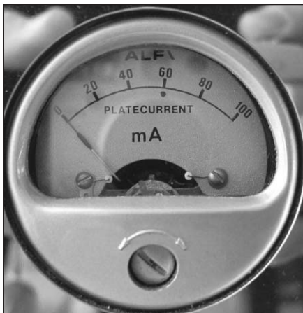
PHOTO 4: Detail meter for the bias of the HQSE 65. The meter originally was a black Russian moving coil type that was re-constructed and re-scaled for measuring plate current. The scale has a tiny red-glowing LED as the 60mA bias point, and is illuminated by two yellow LEDs.
