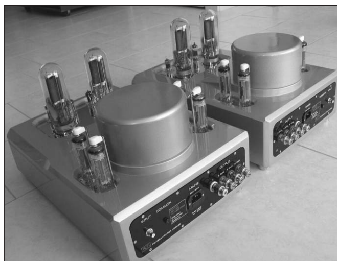
PHOTO 2: A rear view of the two amplifiers, showing the engraved black acrylic back panel with the WBT “Signature” platinum loudspeaker connectors. You can clearly see the large OPTs and the four rectifier tubes.
