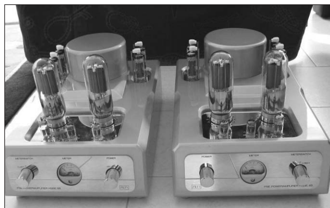
PHOTO 3: The front of the amplifiers shows the 24-carat gold-plated metal plate, engraved with inscriptions and my ALFI logo. The meter is switchable for the left 211, zero, and the right 211. Bias set is 60mA by 1250V DC for the 211s. One of the knobs includes a yellow LED status indicator.
