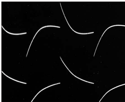
PHOTO 7A: Woofer square-wave responses. Upper trace = uncompensated, lower trace = compensated. 40Hz.
