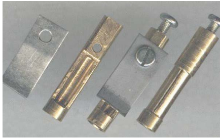
PHOTO 4: Socket pin inserts made on a lathe.
