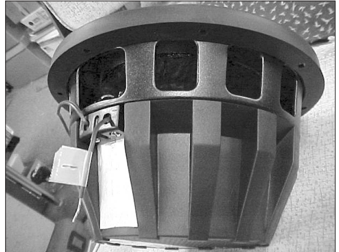
PHOTO 5: View of MA-Audio MA80XE (#196) driver showing near vertical side openings.
