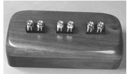
PHOTO 16: Connector block with posts installed.
