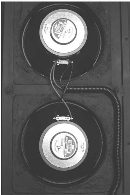
PHOTO 25: Wiring of one driver pair.
