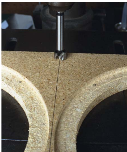
PHOTO 6: Drilling recesses for the mounting bolts.
