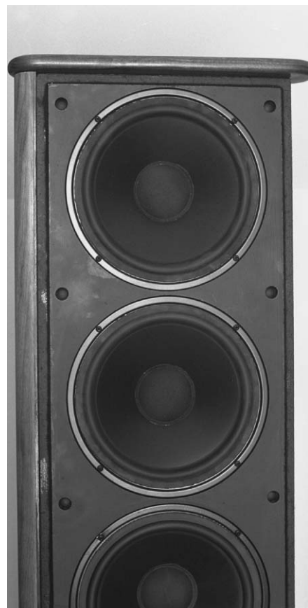
PHOTO 28: Top front of completed speaker without grille.
