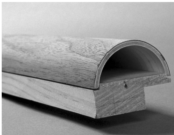
PHOTO 20: Fit of end piece to support.
