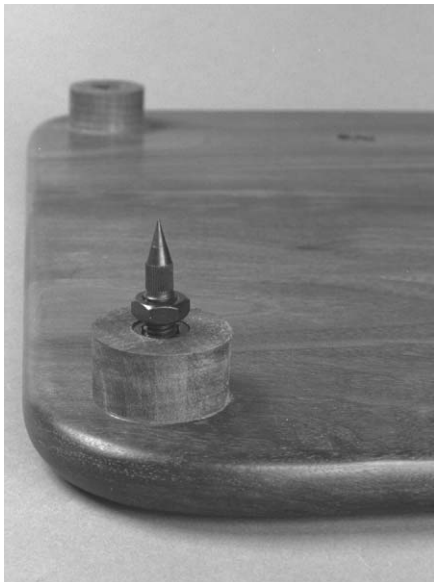
PHOTO 24: Spike inserted into the base.
