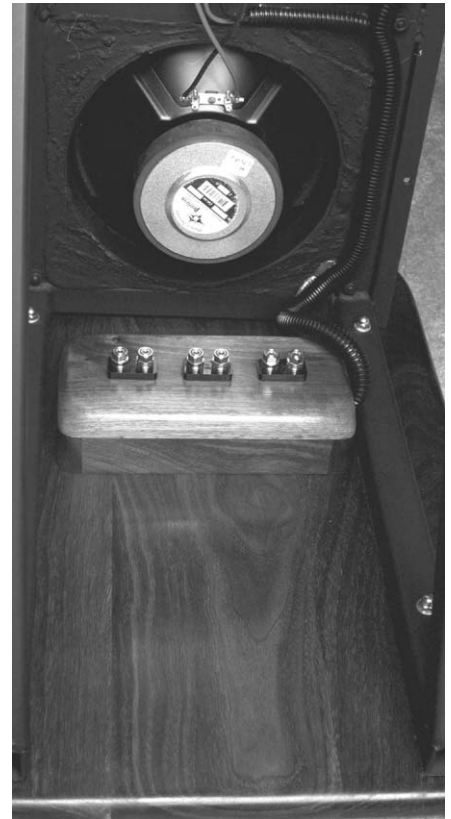
PHOTO 27: Terminal blocks fastened to the base.
