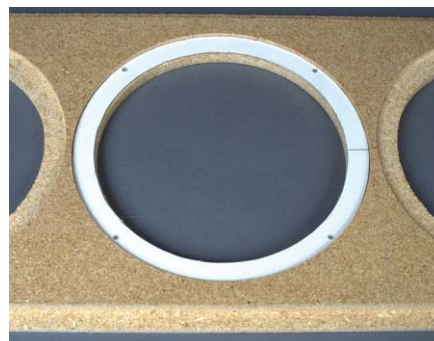
PHOTO 5: Driver drilling template in place.
