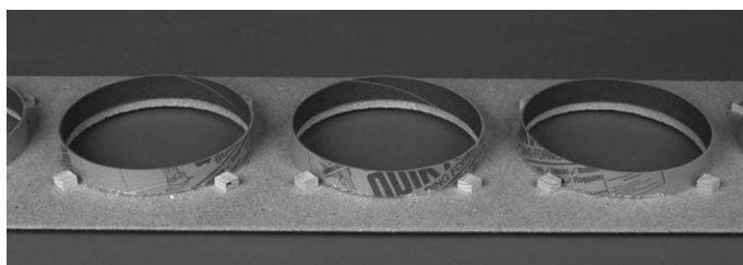
PHOTO 8: Rings installed on the back of the front plate.
