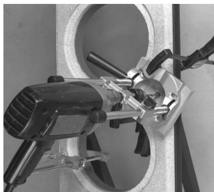
PHOTO 11: Using the front plate as a drilling template.
