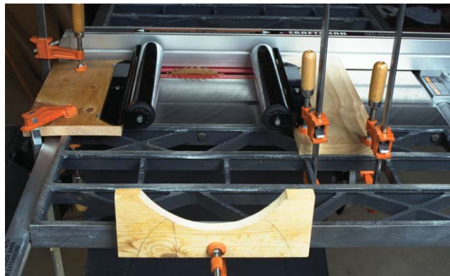
PHOTO 7: Saw setup to cut cement dams.
