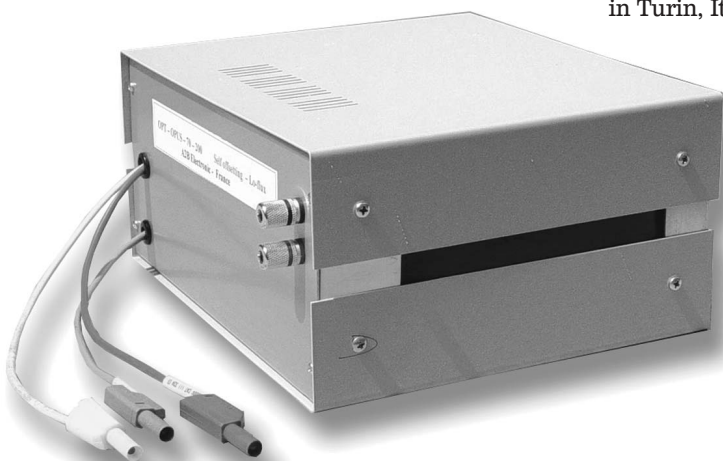
PHOTO 3: The separate power supply box includes the heavy parts that would tremendously increase the cabinet's weight, if located on the main chassis. The white and black cables bring the pulsating rectified DC to the main chassis, for further filtering. Plugs and sockets are of the safety type, with no bare points that could cause electrical shocks.
