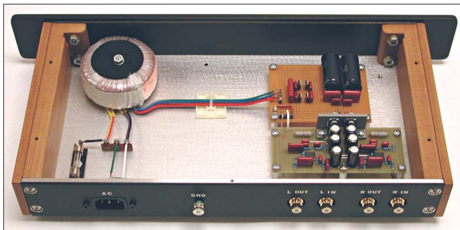
PHOTO 3: Rear overall view of preamplifier.
