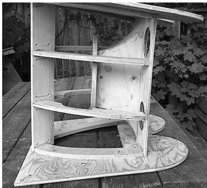
PHOTO 15: The baffle and horn supports installed.
