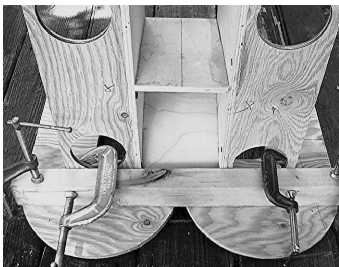
PHOTO 13: Using a guideboard and clamps to hold and align parts for jointing.
