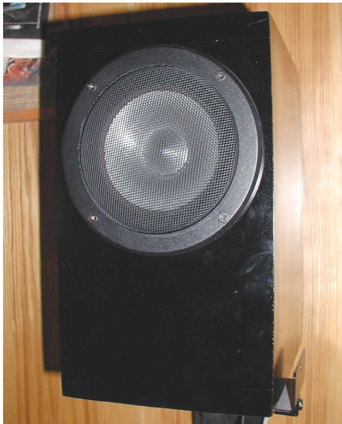
PHOTO 4: Closed box speaker featuring the Jordan JX92S driver.
