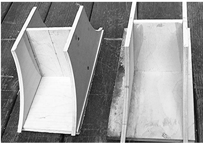
PHOTO 6: Two throat horns on jigs, ready to sheath.
