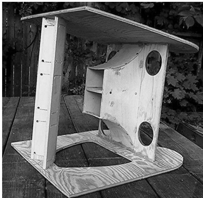
PHOTO 14: Throat horn and tweeter baffle attached to the top and bottom.
