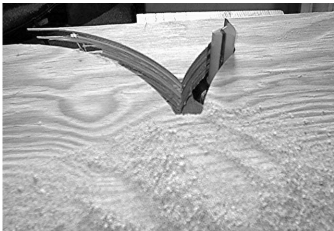
PHOTO 10: Using a router for the radius cuts on the back of the cabinet top and bottom.
