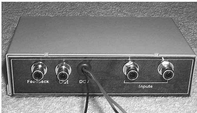
PHOTO 8: Subwoofer filter/controller rear view.
