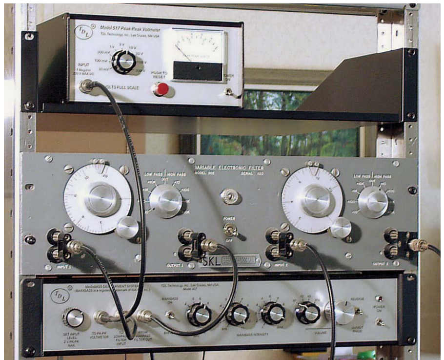
PHOTO 2: MaxxBass test system showing the peak-to-peak voltmeter, dual tunable filter, and the Model 907.
