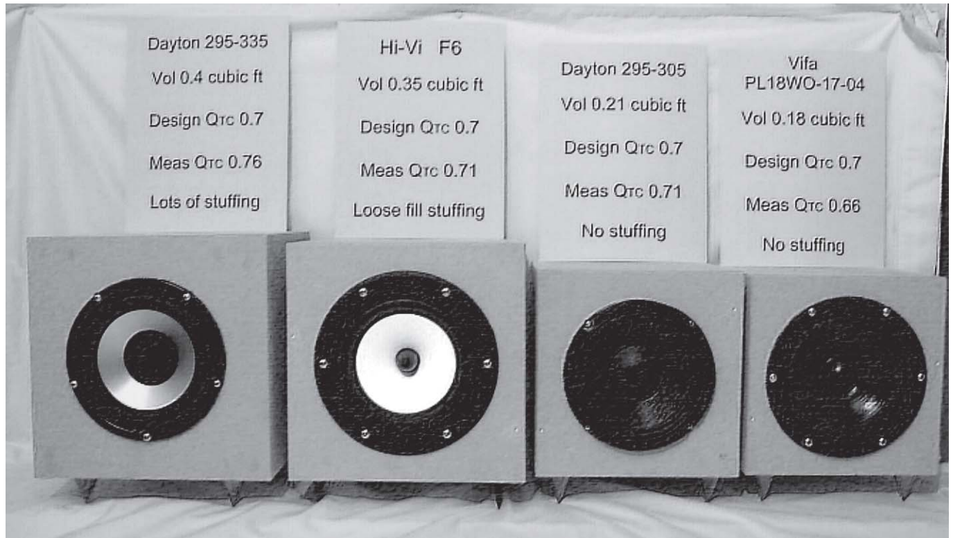
PHOTO 4: The four MaxxBass test speakers. All have a measured closed box Q close to 0.7 9 .
