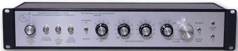
PHOTO 1: Model 907 front panel. Signal in and out connectors and DC power in connector are on the rear panel.
