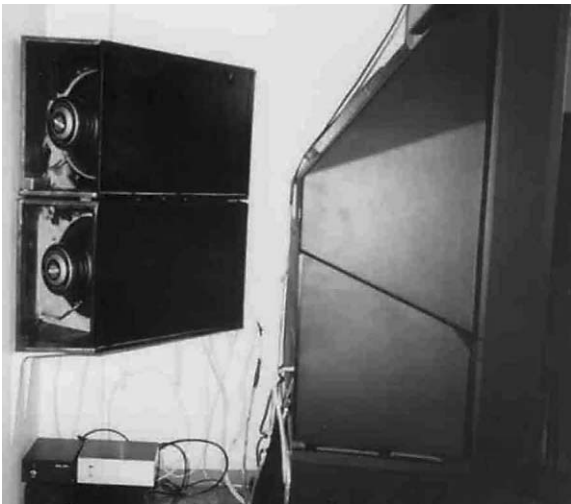
PHOTO 3: Subwoofer installed on the corner of the listening room with the equalizer and the power amplifier below.
