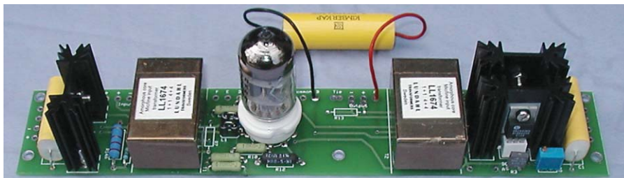
PHOTO 2: A single channel of the differential parafeed line stage.
