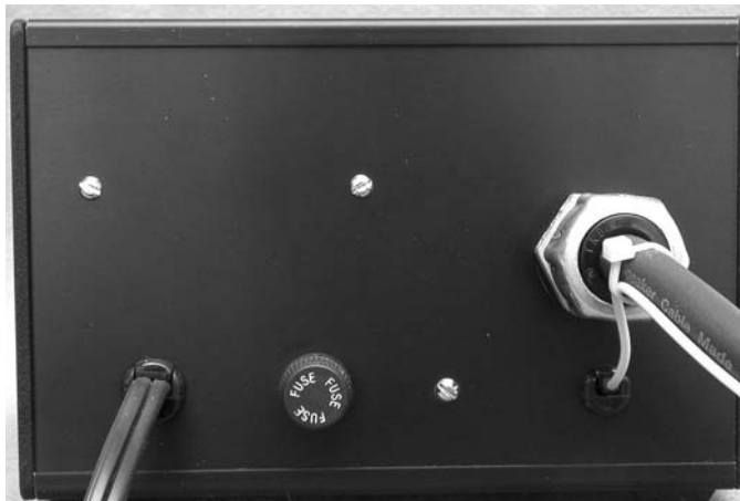
PHOTO 5: Rear panel of the external supply, showing the main DC cable, bias supply wire, AC fuse holder, and AC power cord.
