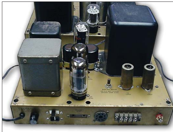
PHOTO 1: The rebuilt Heath W-5M amp.
