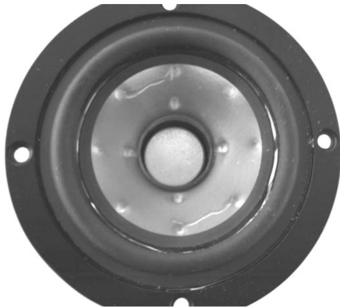
PHOTO 1: Backlit view of front of diaphragm with dust cap removed. The photo shows dimple and glue line placement. With driver mounted in enclosure, the glue lines are not visible.
