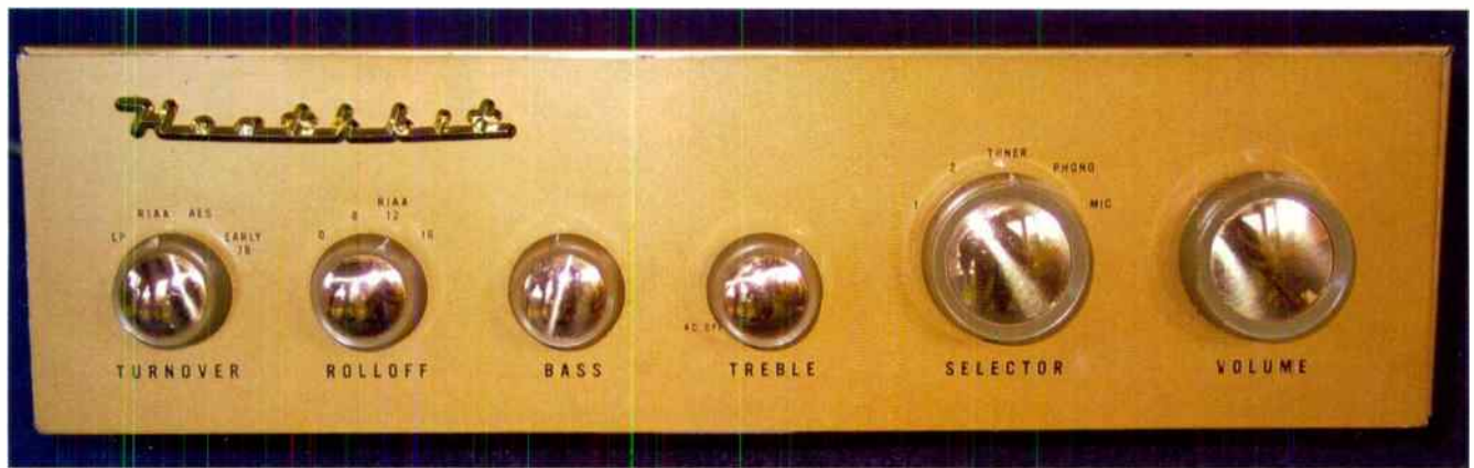
Figure 2: A recently purchased WA-P2 preamp shows the basic functions. And it doesn't look bad for being nearly 50 years old, after cleanup with just soap and water!
