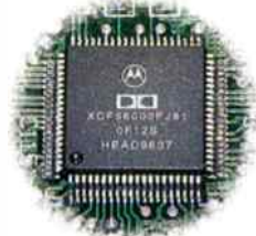
B&K's new surround sound components are powered by the 24-bit Motorola 56000 DSP.
