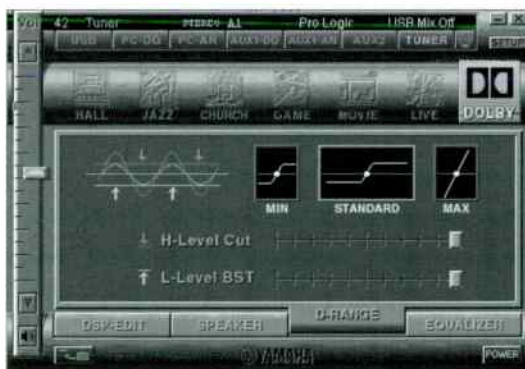
The D-Range control can help keep signals with wide dynamic ranges from overwhelming your ears.
