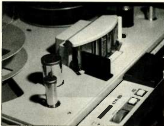
A typical test jig, shown here on a Tascam ATR-80 24-track recorder.
