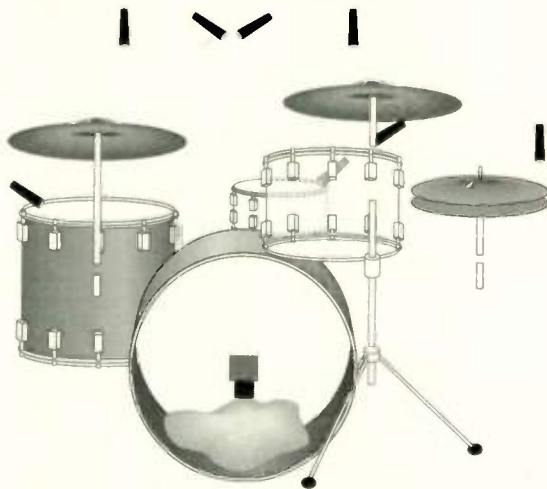
Basic mike placement for a drum kit. Two overhead options are shown: placed wide, or pointed together in an XY stereo configuration.
