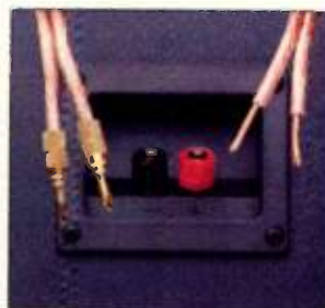
The Monitor One's five-way binding posts accept even extra-large monster size, banana plugs and spade jags. Hookup is fast, easy and reliable.
