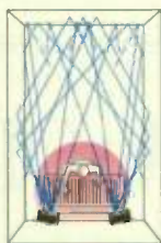
The pink area in the illustration shows where direct sound energy overpowers reflected waves in a typical mixing room. The Monitor One helps eliminate such complex acoustic problems by focusing direct sound energy toward the mixing position.
