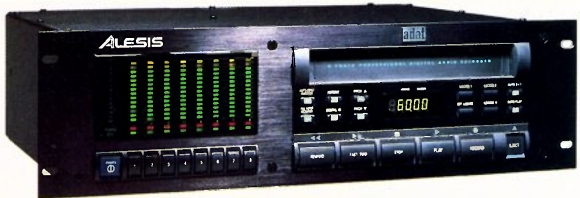
MORE TIME WITH LESS TAPES: With the new software, ADATs can now use T-180 tapes.
