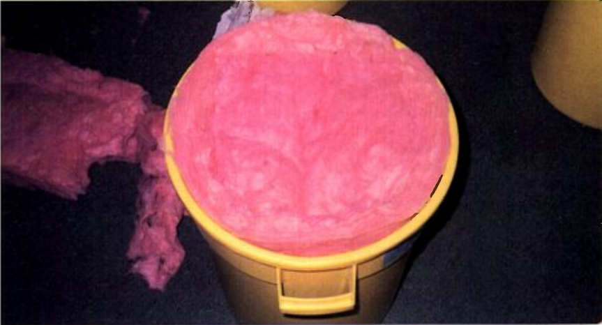
FIGURE 5: After placing the two vertical pieces of fiberglass, place another piece on top.
