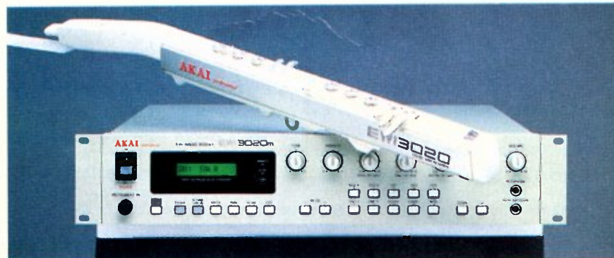
EWI, EWI, OH: An Electronic Wind Instrument (EWI), like Akai's EWI3020 above, can introduce a variety of familiar and unique sounds to your recordings.
