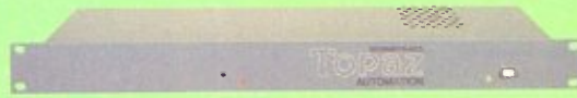
No external fader bays, no insert points used, a completely seamless installation with the Topaz Automation Controller Unit, (TACU), interfacing between console and PC.
