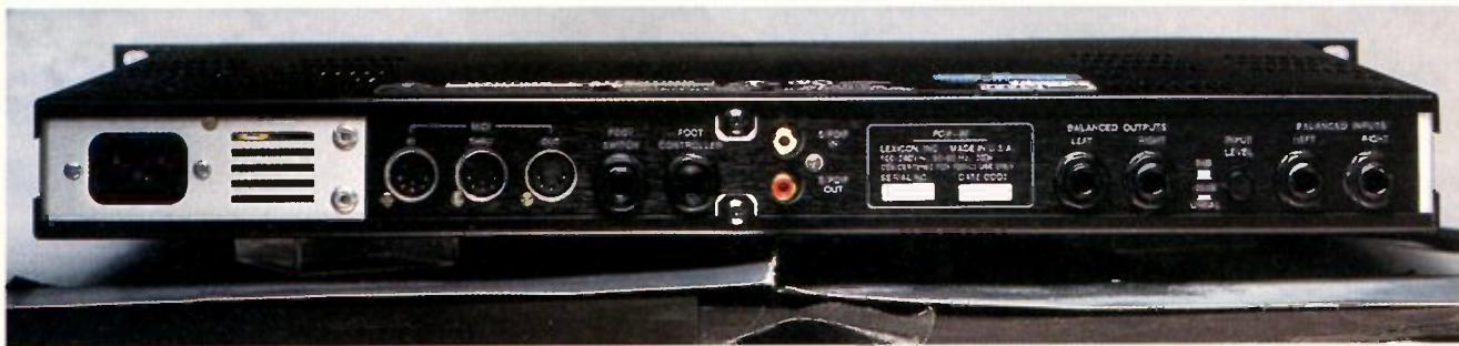
BACK TO THE FUTURE: The PCM 80 includes both analog and digital I/Os for whatever format you work in (or plan to work in).
