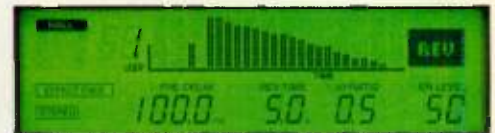
Turn the reverb time control, see the reverb time displayed graphically.
