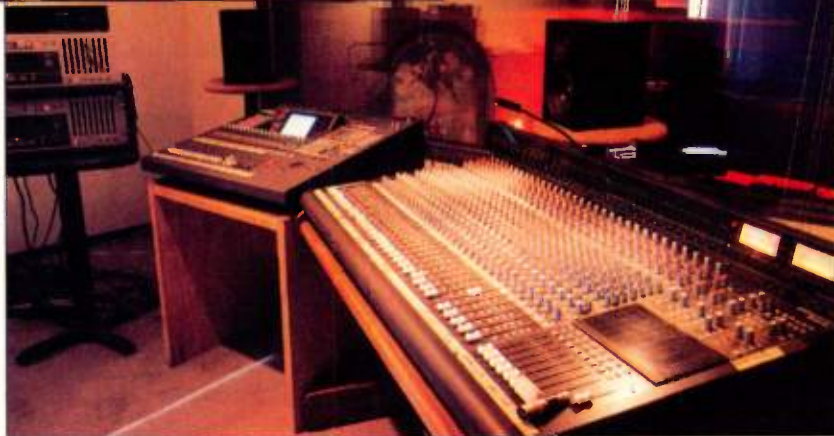
THE BOULDER & THE BEAUTIFUL: The recording booth features a 32-channel Mackie 8•Bus, Yamaha 02R, and TASCAM DA-88's.
