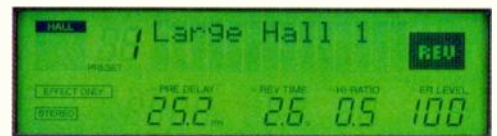
Large LCD display shows effect type, name and current settings.
