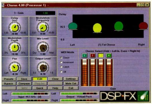
FIGURE 1: The DSP•FX Chorus screen. Note how the graphics indicate relative delays and extent of modulation.
