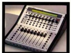
The Motor Mix is the only DAW control surface to offer eight 100-mm longthrow motorized faders, configured into a series of eight switchable banks.
