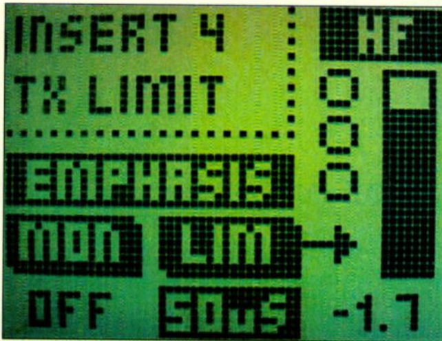
FIGURE 3: Using the high-frequency emphasis along with its dedicated limiter to improve intelligibility.
