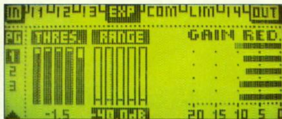
FIGURE 2: Threshold, Release, Range, Ratio, and more can be independently set for each band.
