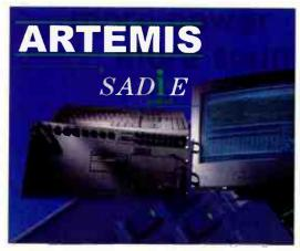
rack mounting turnkey systems in a range of input/output configurations, from 8 to 24 inputs and outputs. The entry-level ARTEMIS system is equipped with 8 inputs and 8 outputs, and can replay 24 tracks of edited 16-bit audio. Twenty-bit analog conversion is built into the system and external converters are provided for by AES/EBU digital I/O on every channel. For additional information, contact SADiE, Inc. at 615-327-1140. Circle EQ free lit. #112.
