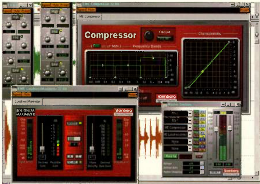
FIGURE 1: This setup was the starting point for most of the tunes with vocals. The multiband compressor brought up the vocal intelligibility somewhat while leaving the rest of the track unaffected.
