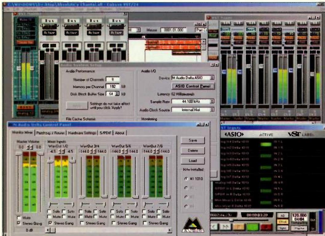
FIGURE 1: The 1010 software mixer used with Cubase. Toward the lower right of the screen shot, note the window that shows which inputs are available to Cubase.
