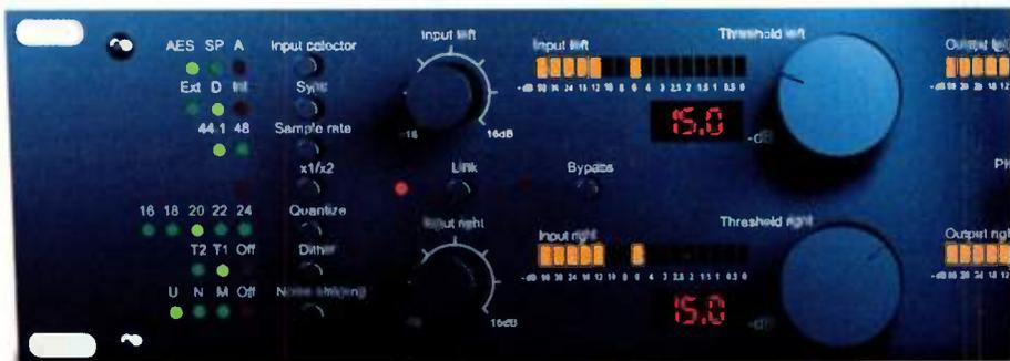
it's difficult to duplicate settings or to match the two channels. Even more problematic, the input trim knobs on my review unit weren't lined up; one pointed several degrees off from the other. I pulled the knobs off and attempted to re-seat them, but was unable to completely align their markings. It's possible that you could open the box and physically twist the potentiometers to line them up, but, on a box intended for pro mastering, this shouldn't be necessary.
