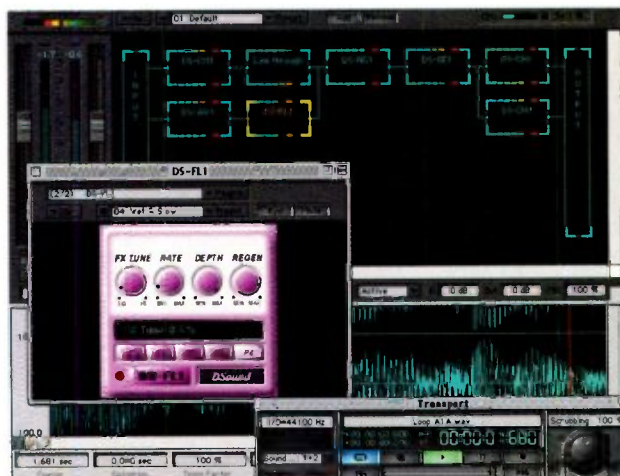
FIGURE 2: Several plug-ins loaded in Spark's FX Machine. The flanger is highlighted; it's in "small" graphics mode, as opposed to the "normal" mode evidenced in fig. 1. Note how two choruses are placed in parallel at the output. The CPU indicator shows 34.1% — pretty good for seven plug-ins.
