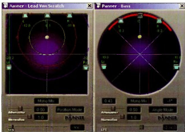
FIGURE 5: NUENDO'S SURROUND PANNER (TECHNICALLY IT'S A PLUG-IN, BUT IT FUNCTIONS TRANSPARENTLY AS PART OF THE MIXER) CAN OPERATE IN EITHER OF TWO MODES: POSITION (ABOVE LEFT) OR ANGLE (ABOVE RIGHT). BOTH ARE USEFUL, DEPENDING ON WHAT YOU'RE TRYING TO DO; "POSITION" IS BETTER FOR PLACING A SOUND IN THE SOUNDFIELD. IN THE PANNER ON THE LEFT, I'VE BROUGHT THE LEAD VOCAL OUT INTO THE FIELD A BIT, WHICH HELPS ITS PRESENCE IN THE MIX.
