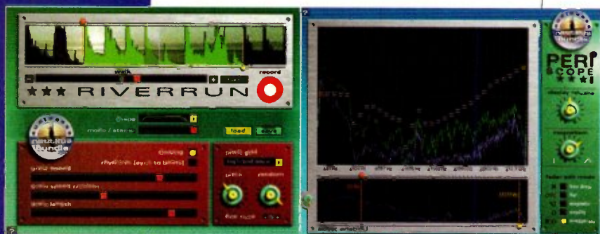
FIGURE 1 (left): RiverRun is a unique plug-in; the first to offer granular synthesis. FIGURE 2: Periscope offers a low-pass and a high-pass filter, as well as 30 band-pass filters in a highly controllable package.
