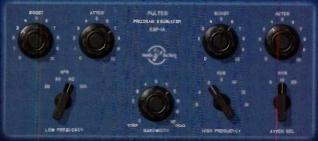
The Pultec equalizer provides smooth, sweet EQ and an extremely high quality tube audio signal path. Use Bomb Factory's meticulously-crafted replica anywhere you'd use the original: on individual tracks, critical vocals, or even across a stereo mix for mastering applications.
