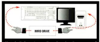
You don't have to go through a lengthy process of converting files to get them between the MX-2424 and Pro Tools. Just record onto a removable SCSI drive with your MX-2424, then pop it into your Mac or PC. Your DAW system will open the files just as if they'd been originally recorded on the computer.
