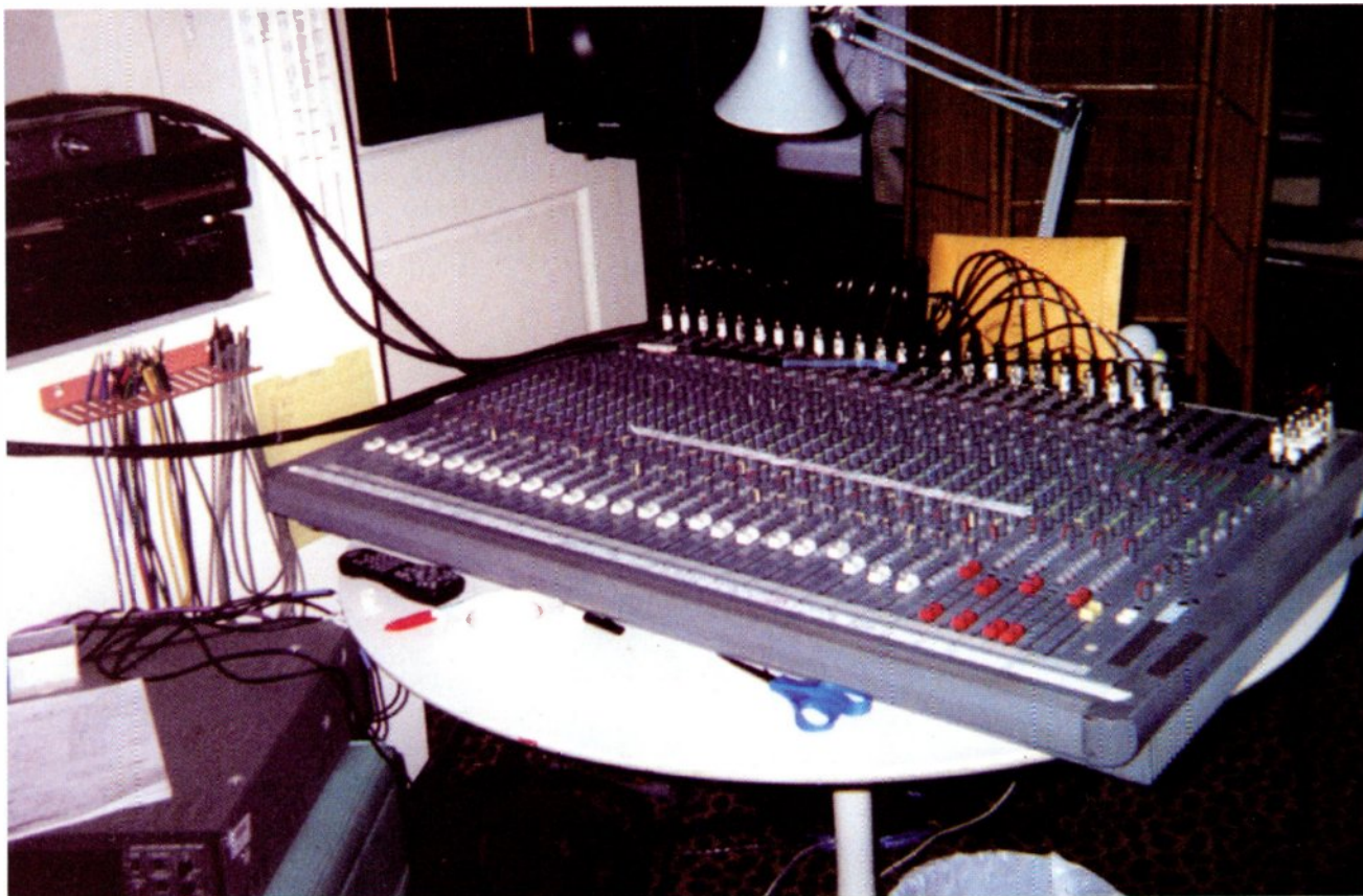
Once the recordings were finished, the mixes were done on a Soundcraft Spirit Studio console.
