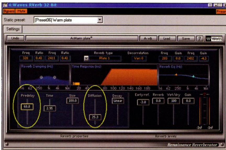
FIGURE 5: The reverb in the RVerb plug-in from Waves offers an exceptional amount of control. Note the diffusion and predelay parameters, which are circled in yellow.
